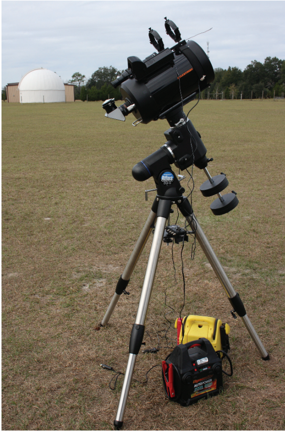
Plate 10. (German mount) A C8 CAT mounted on Orion's Atlas EQG German equatorial mount. Credit: Author.
