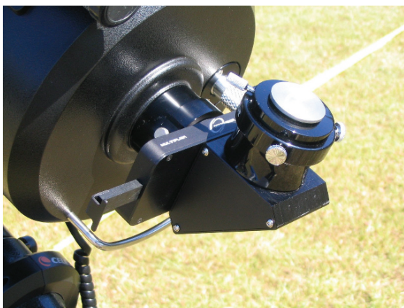
Plate 42. (Denkmeier Powerswitch) The ultimate star diagonal? Denkmeier SCT Power-switch diagonal. Credit: Author.
