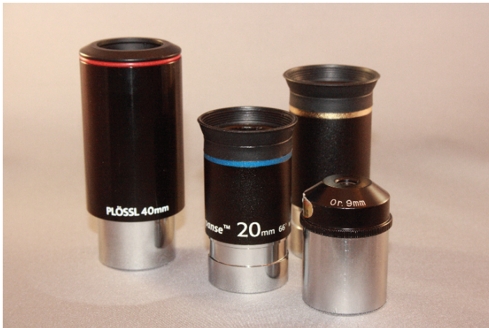
Plate 36. (Narrow/Medium Field Eyepieces) A collection of narrow to medium field eyepieces, (l-r) Pro-optic 40mm Plössl, Orion Expanse 20mm, Orion Expanse 9mm, Celestron 9mm Orthoscopic. Credit: Author.
