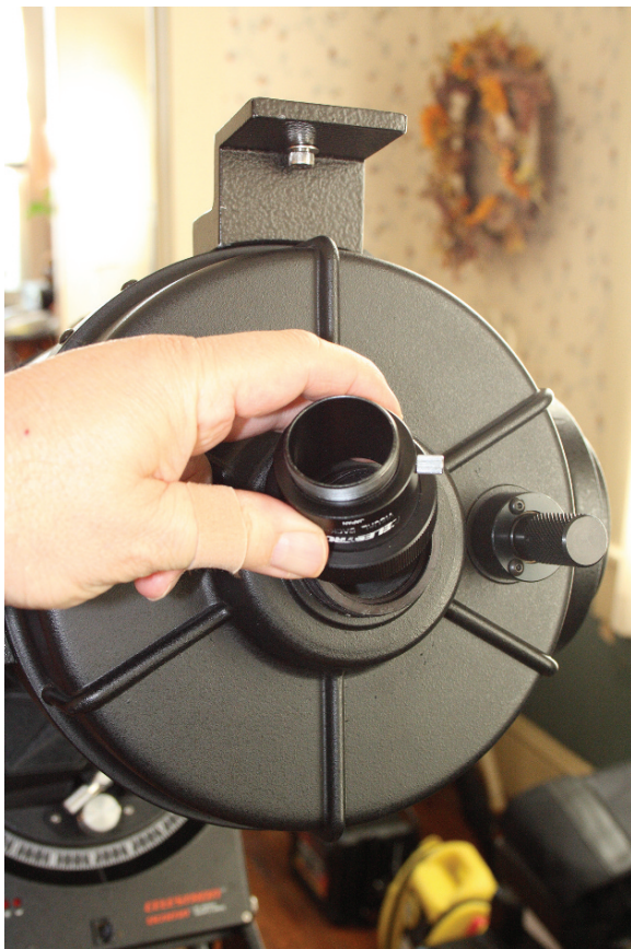
Plate 7. (Rear Cell) SCT rear cell assembly showing rear port, visual back, and focus knob.” Credit: Author.
