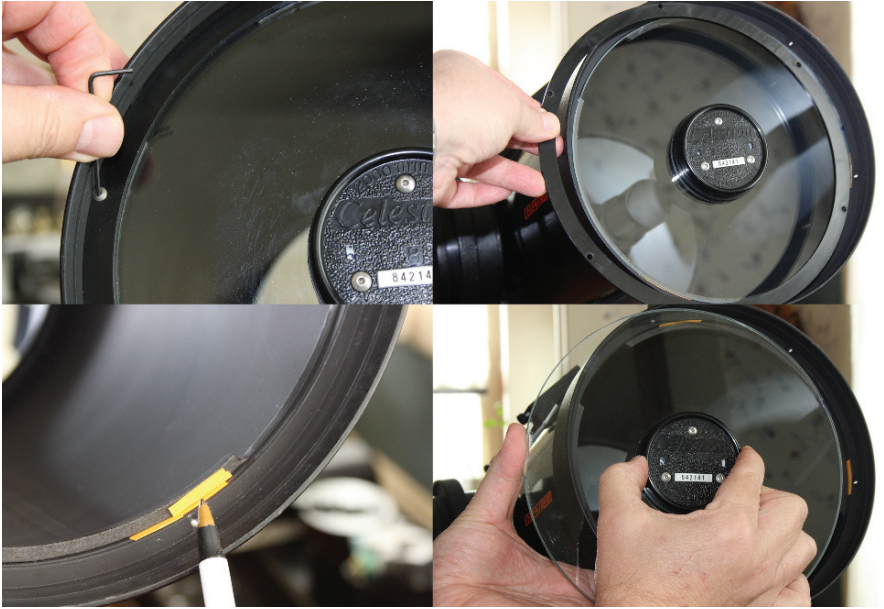
Plate 60. (Pulling a Corrector) Clockwise from upper left, (a) unscrew Allen head screws, (b) remove the retaining ring, (c) hold onto the secondary mount and pull the corrector out, (d) carefully note the positions of paper shims.
