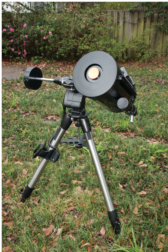
Plate 35. (Balancing a GEM) Good balance is important for accurate GEM go-to and tracking, but is easy to achieve. Credit: Author.
