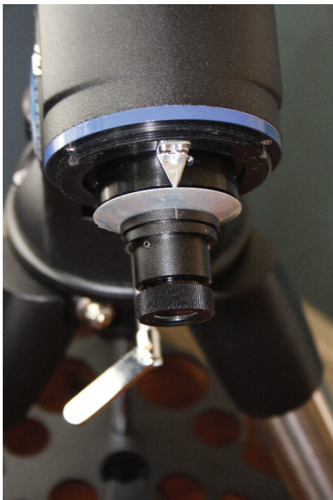
Plate 48. (Polar Scope) The eyepiece end of a German equatorial mount's polar alignment borescope. Credit: Author.
