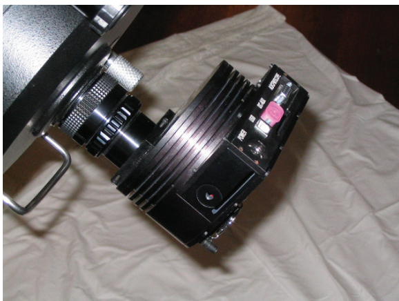
Plate 75. (SBIG ST2000) SBIG's ST2000 CCD camera offers both a generous-size imaging chip and extreme sensitivity. Credit: Author.
