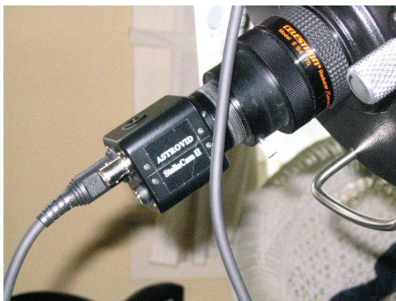
Plate 78. (Stellacam II) The small but sensitive Stellacam II deep sky video camera is able to provide near real time images of deep space objects. Credit: Author.
