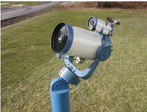
Plate 3. (Blue and White Celestron) One of the Celestron's legendary 1960s Blue and White SCTs, the C10. Credit: Image courtesy of Bob Piekriel.
