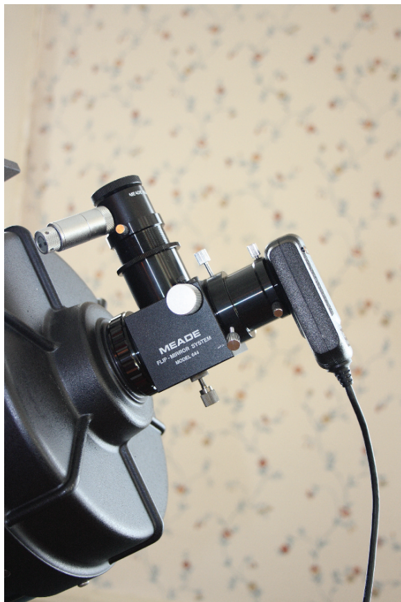
Plate 71. (Meade 644 Flip Mirror) A flip mirror like Meade's model #644 makes it easy to center planets on tiny webcam chips. Credit: Author.
