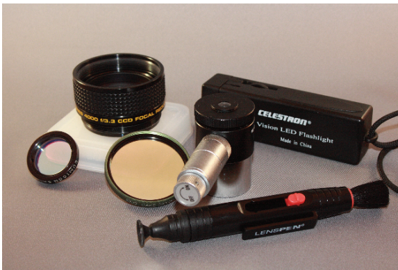
Plate 39. (Assorted Accessories) A few of the accessories amateurs find themselves constantly buying, (l-r) Lumicon UHC LPR filter, Celestron f/6.3 reducer/corrector, Thousand Oaks OIII LPR filter, Meade 12mm illuminated reticle eyepiece, Lenses, Celestron LED astronomer's flashlight. Credit: Author.
