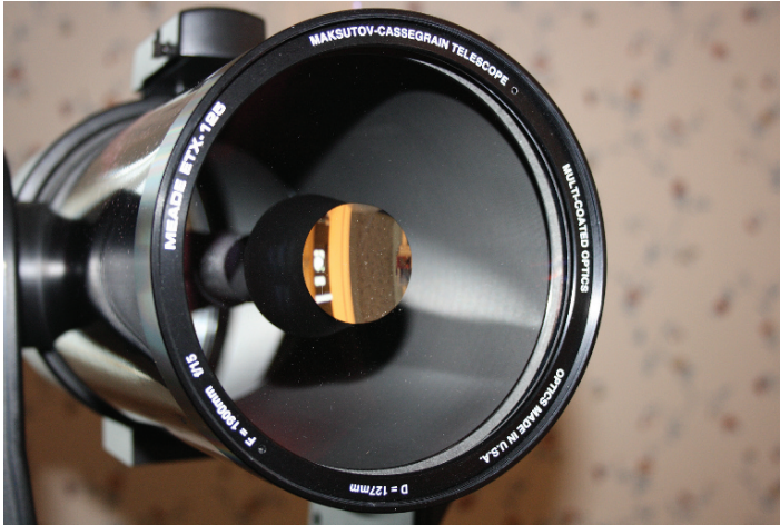
Plate 12. (MCT Corrector) The deep-dish corrector plate of a Gregory-style Maksutov Cassegrain telescope, the Meade ETX125PE. Credit: Author.
