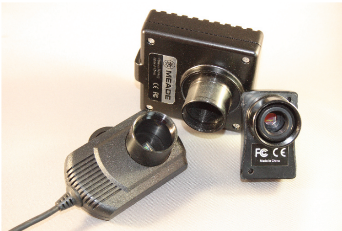
Plate 70. (Webcams) Webcams and webcam like imagers can shoot everything from the Moon to the most distant galaxies. L – r: Celestron NexImage, Meade Deep Space Imager (DSI), Meade Lunar and Planetary Imager (LPI). Credit: Author.
