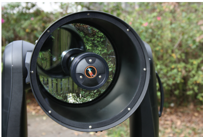
Plate 34. (Corrector End of a CAT) Looking down the front of a Celestron NexStar11 GPS. Credit: Author.
