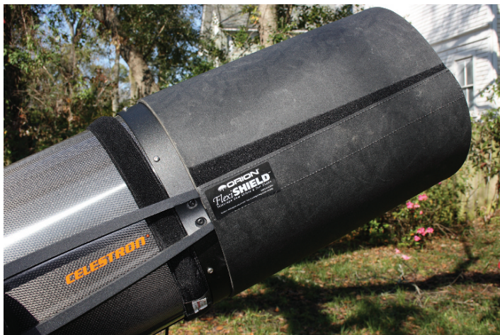
Plate 46. (Heater) Correctly positioning a dew heater strip behind the corrector assembly is important for good performance. Credit: Author.
