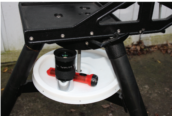
Plate 82. (Accessory Tray) Many SCT tripods lack handy accessory trays. This can be rectified at almost no cost with the lid of a 5-gallon paint bucket. Credit: Author.
