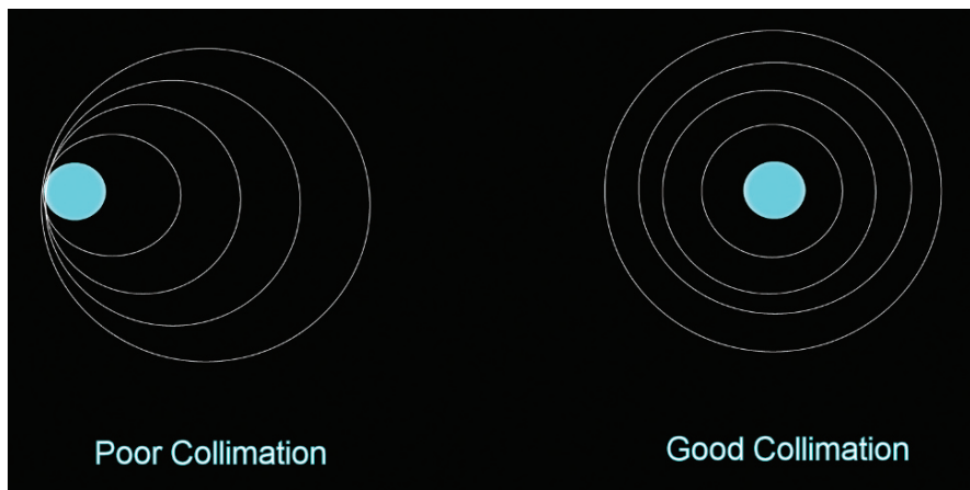
Figure 6. (Fine Collimation) If the ‘bull’s-eye’ diffraction rings are not concentric, there’s collimating to do!
