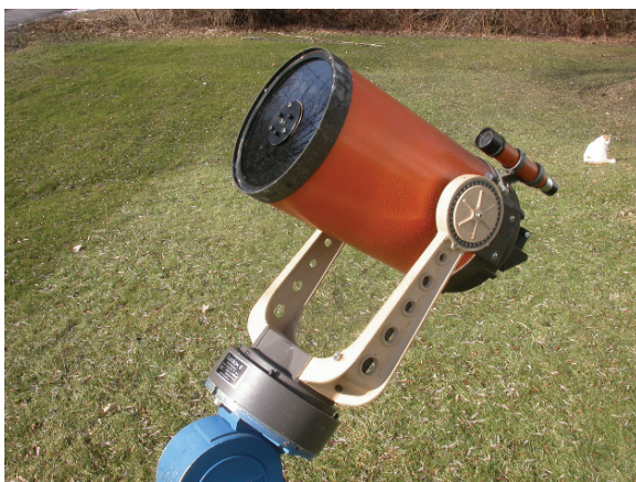
Plate 4. (Orange Tube Celestron) Celestron’s first mass produced Schmidt Cassegrain, the ground-breaking Orange Tube C8. Credit: Image courtesy of Bob Piekieł.
