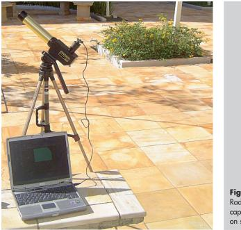
Figure 2.58. PST and RadioShack webcam capturing a PST image on screen.
