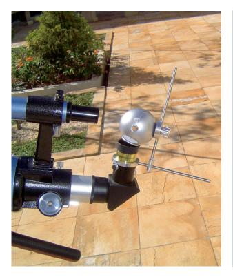
**Figure 2.57.** Afocal camera adaptor with Coronado CEMAX eyepiece.
