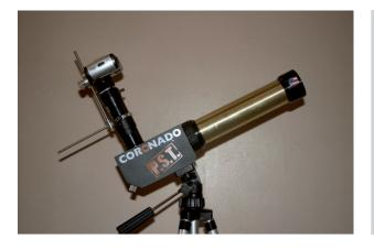
Figure 2.51. PST with afocal adaptor.
