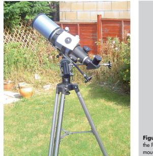
**Figure 2.9.** Mounting the PST on an equatorial mount, sequence 1.
