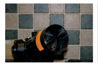
**Figure 5.47.** Baader filter fitted to a Meade ETX90.
