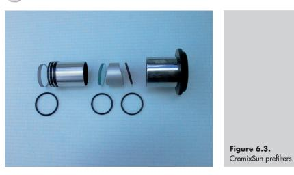
The units are placed near the end of the light path from the objective. They use standard 1.25-inch connections and have an infrared blocking filter.
