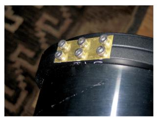
Figure 3.5. T-Max ring attached between the filter and the telescope. Photo by Larry Alvarez.
