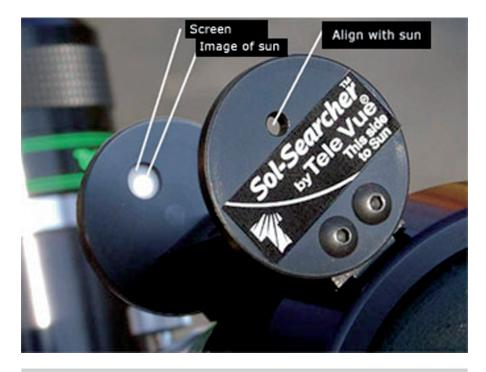
Figure 7.9. Sol Searcher. Courtesy of SolarScope.
