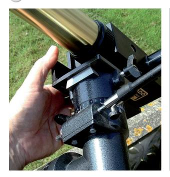
**Figure 2.17.** Mounting bracket for the PST Part 6: Fitting the PST to the mount. Courtesy of John Watson.
