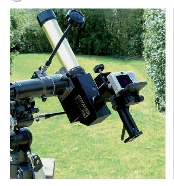
**Figure 2.54.** Canon Powershot SD450 mounted with the PST.
