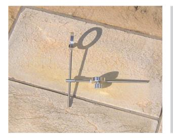
Figure 2.56. Afocal camera adaptor.
