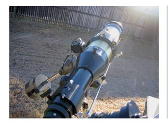
**Figure 3.3.** MaxScope 90 showing the clamshell with the Sol Ranger on top. Photo by Larry Alvarez.
