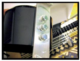
Figure 3.4. Lower view of clamshell with tripod attachment. Photo by Larry Alvarez.
