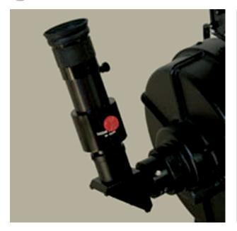
Figure 7.15. Thousand Oaks hydrogen alpha unit attached to a telescope. Courtesy of Thousand Oaks Optical.
