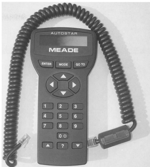
Figure 3.13. Autostar computer controller.
