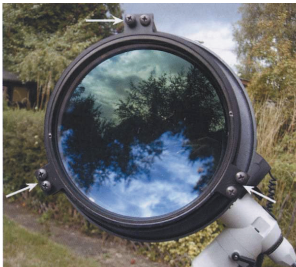
Figure 11.2. AR-6 primary lens collimation screws.
