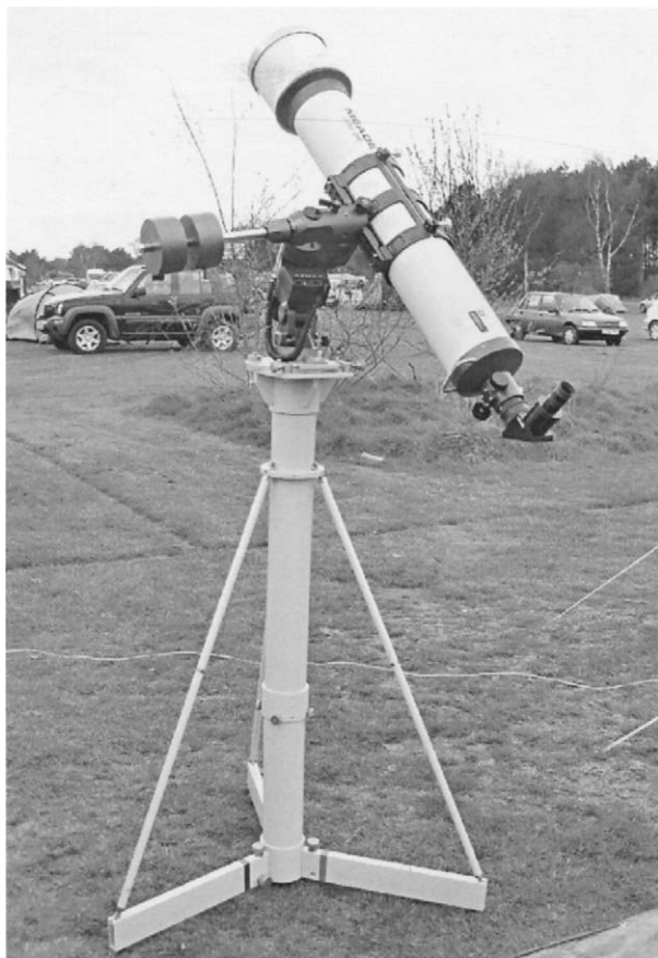
Figure 3.7. Typical pillar stand. Image courtesy of Alan Marriott.
