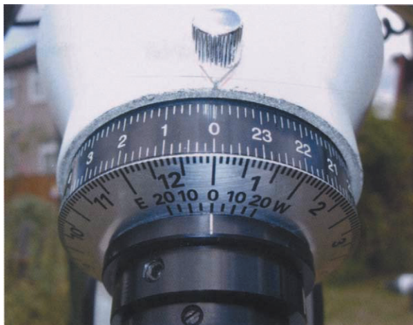
Figure 5.6. RA setting circle and calendar dial.
