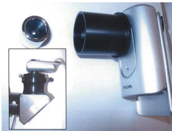
Figure 10.6. ToUcam Pro with prime focus adaptor and shown fitted to telescope (inset).
