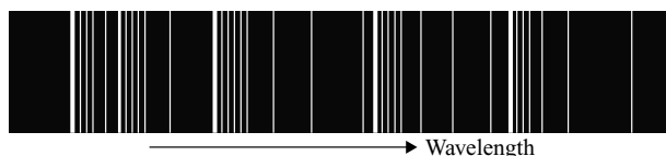
Figure 7.11. A stylised (and very much simplified) electron vibration rotation transition series (i.e. a molecular band). The thicker lines represent the head of each vibration rotation series, which themselves also get closer towards shorter wavelengths to form the molecular band head.
