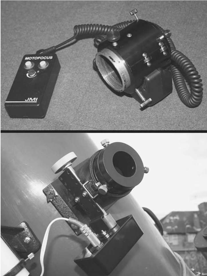
Figure 8.5. Two types of electric focuser: a Crayford-type screw-on micro-focuser for SCTs (top), and a simple motor box added to a standard Newtonian rack-and-pinion focuser (bottom).
