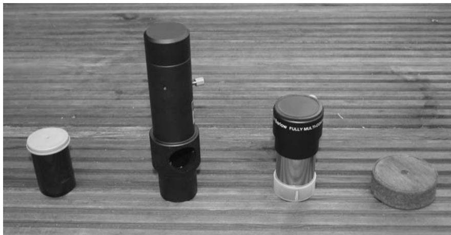
Figure 10.1. Tools for precise Newtonian collimation: drawtube stop (film canister), laser collimator, Barlow, and drawtube inner-end stop.
