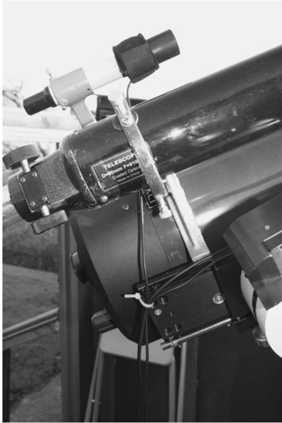
Figure 7.3. Dew-heater cables tied to a mounting plate to minimise problems with snagging the mount.
