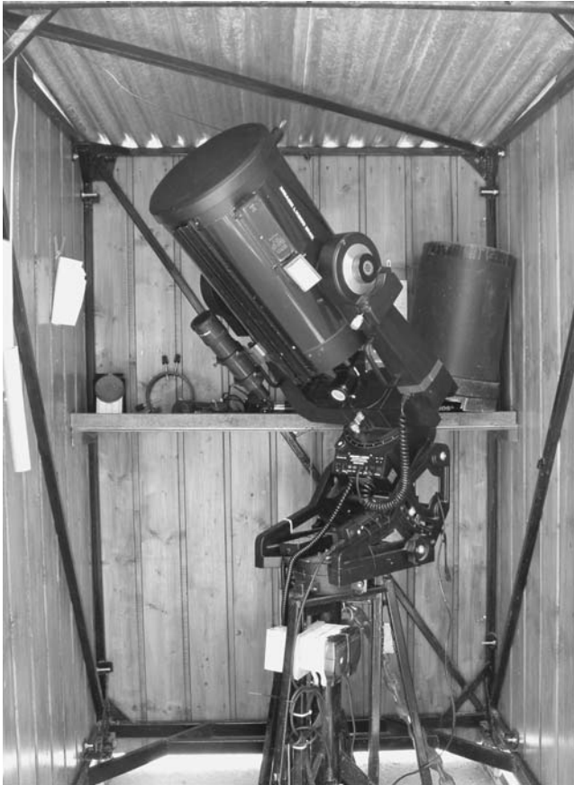
Figure 9.13. The inside of the SCT run-off shed.
