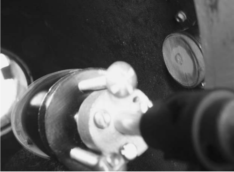
Figure 10.3. Looking into the side of the telescope tube from the front, this shows the ring-shaped shadow of the centre mark produced by the laser and Barlow almost centred on the drawtube faceplate.
