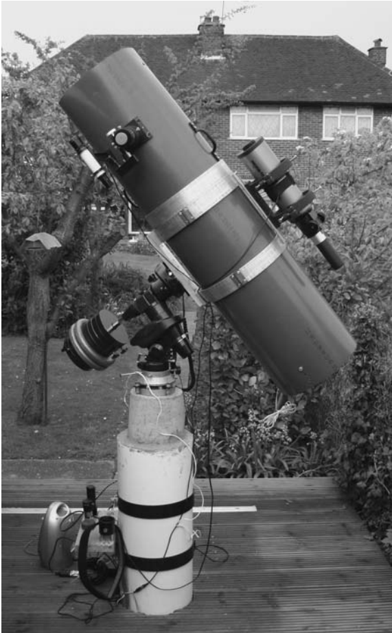
Figure 9.28. The 245 mm f4.8 Newtonian telescope on its concrete and aluminium pier.
