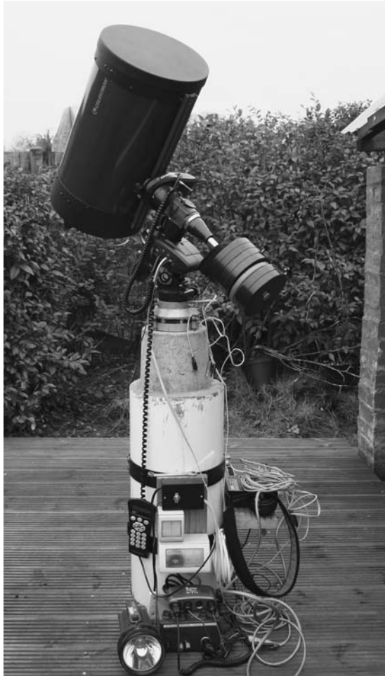
Figure 3.4. With an observatory without fixed walls, wiring and electronics tend to get crowded round the pier.
