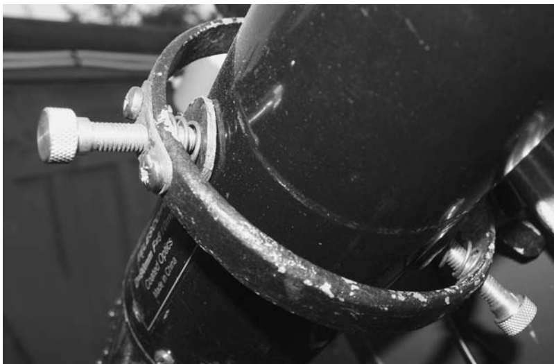
Figure 10.12. Guidescope ring modification with springs and plastic disks.
