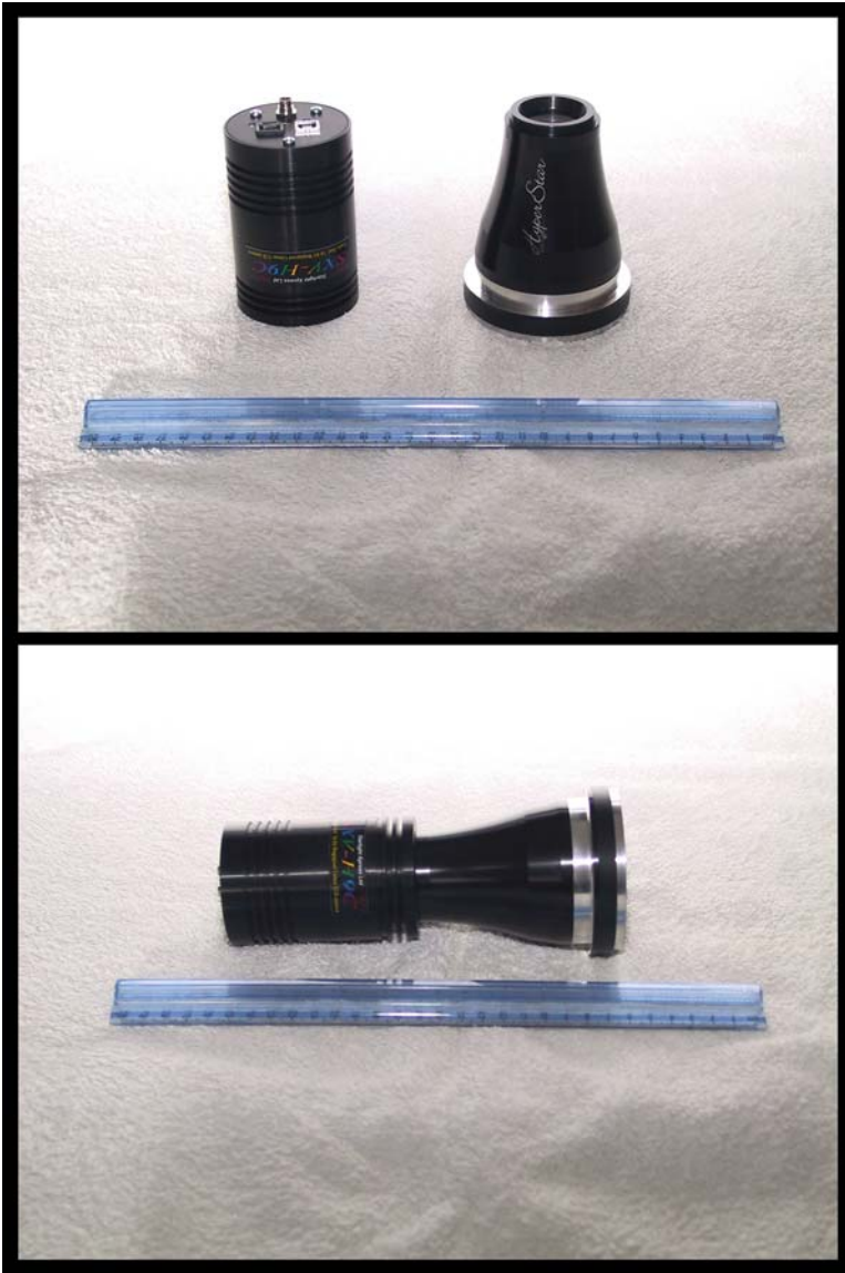
Figure 1.1. The Hyperstar lens assembly and the SXV-H9C one-shot colour CCD camera from Starlight Xpress. Bottom photo – the two elements connected.
