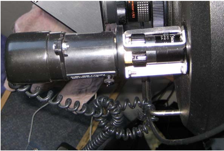
Figure 1.2. The standard Celestron electric focuser, mounted on home-built aluminium standoff pillars, to fit the Starizona “FeatherTouch” focuser.
