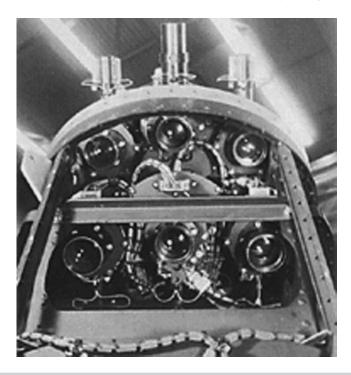
Figure 9.17. Ranger 9's Vidicon Cameras (Credit-NASA).
