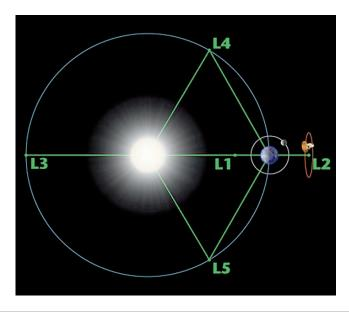
Figure 1.49. Lagrange points (Credit-NASA).
