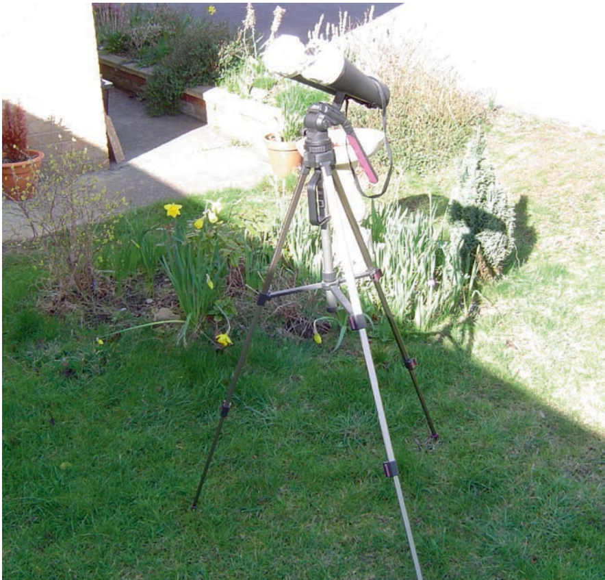
Fig. 3.4. A pair of 15×70 binoculars fitted with white light filters.
