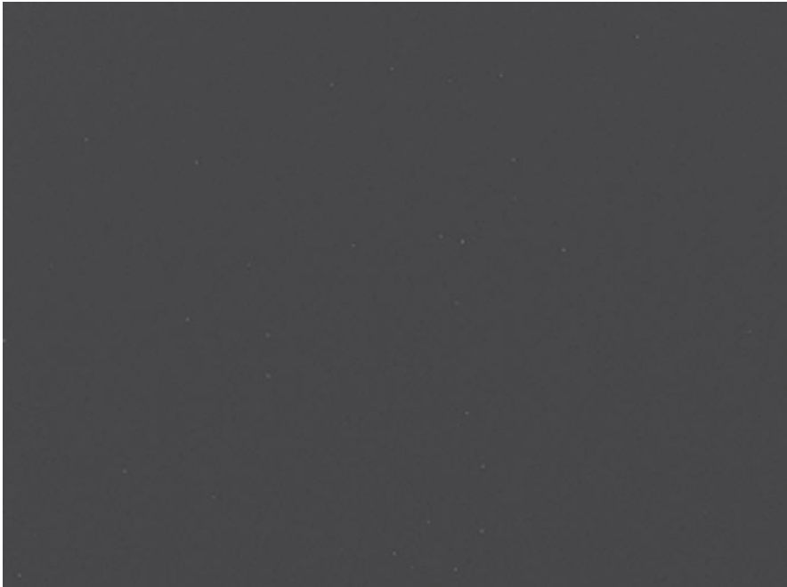
Fig. 9.36 SXV H9 min dark frame at an ambient temp of 15 degrees centigrade.
