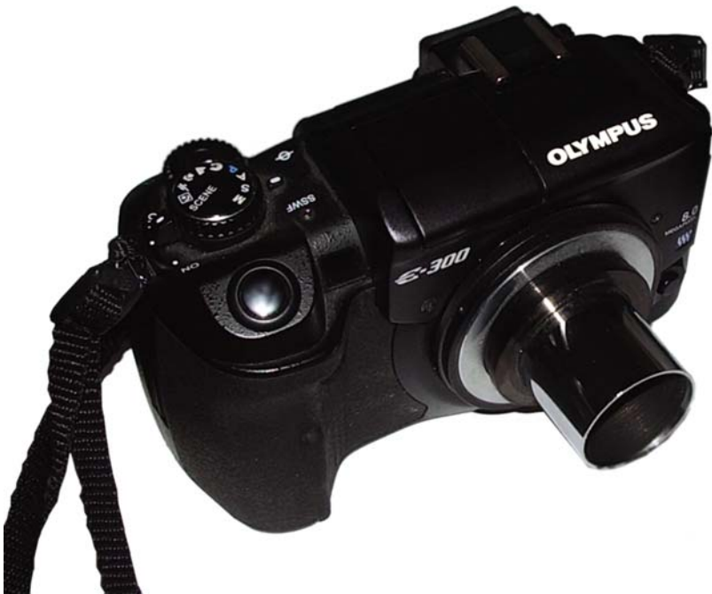
Figure 2.38. The author's Olympus E-300 DSLR, shown with a T-adapter for prime focus imaging through a telescope (photo by Peter Grego).
