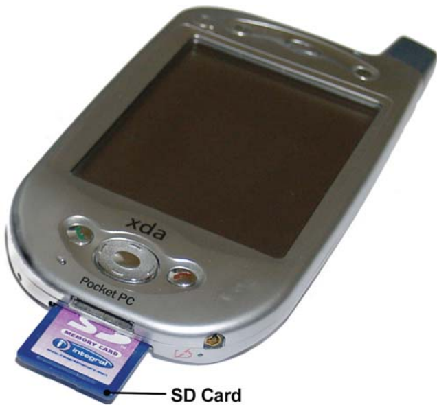
Figure 5.7. The author’s XDA PDA, showing the location of the SD Card at the base of the device (photo by Peter Grego).
