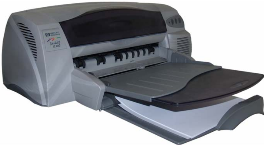
Figure 2.30. The author's A3 format Hewlett-Packard Deskjet 1220C inkjet printer. It uses cartridges with their own print heads (photo by Peter Grego).
