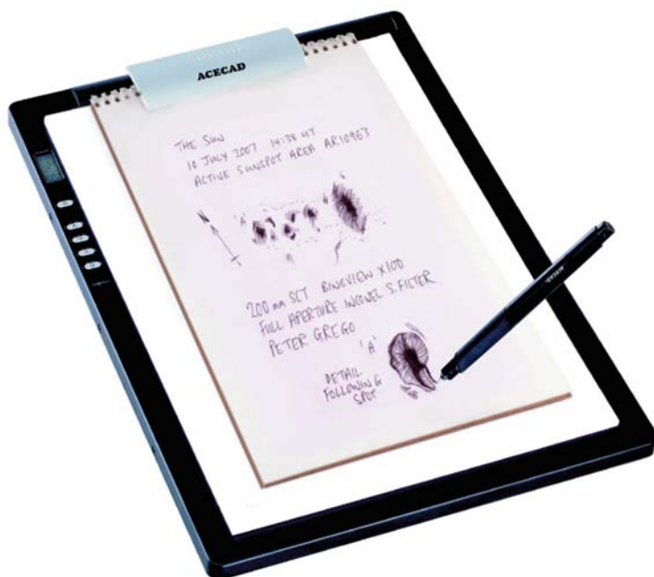
Figure 2.18. A Digimemo A402 digital notepad (showing a simulated astronomical sketch) (photo by Peter Grego).
