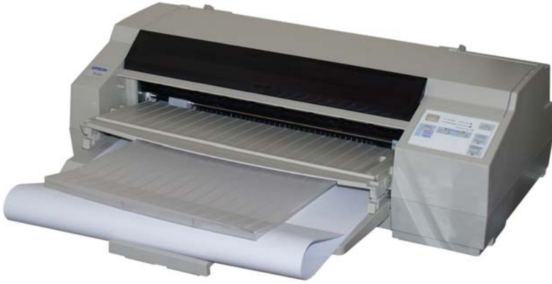
Figure 2.29. The author's large format Epson Stylus Color 1520 inkjet printer has a fixed print head (photo by Peter Grego).
