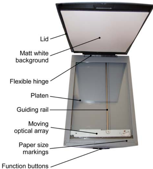
Figure 2.33. Main components of the author's Canon CanoScan LiDE 30, a USB-powered flatbed scanner (photo by Peter Grego).
