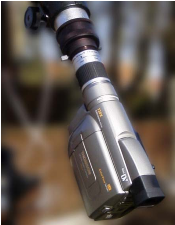
Figure 2.39. A camcorder set up for imaging through the telescope eyepiece (photo by Peter Grego).
