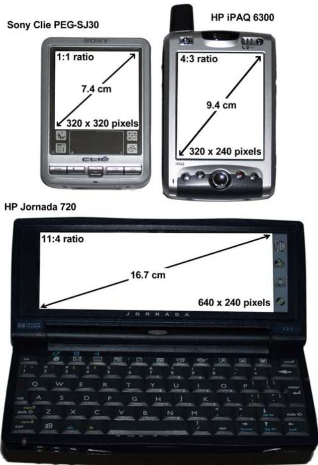
Figure 4.6. Screen formats compared in scale – Sony Clie PEG-SJ30, Hewlett-Packard iPAQ 6300, and Hewlett-Packard Jornada 720 (photo by Peter Grego).
