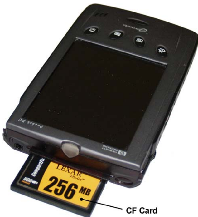
Figure 5.3. The author's Jornada 540 PDA, showing the location of the CF Card at the top of the device, in front of the backup battery (photo by Peter Grego).
