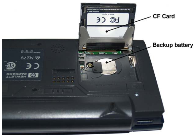
Figure 5.2. The author's Jornada 720 handheld computer, showing the location of the CF Card at the base of the device, in front of the backup battery (photo by Peter Grego).
