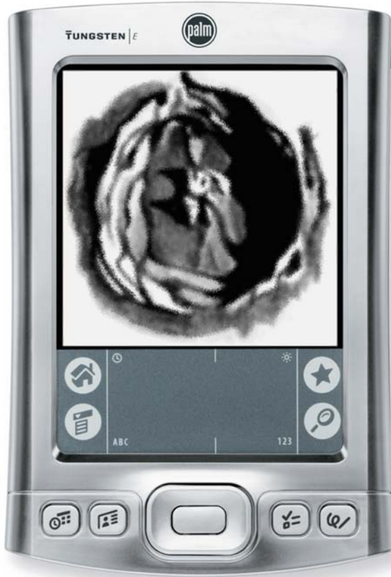
Figure 4.4. A Palm Tungsten E PDA, showing the square LCD touchscreen and the Graffiti scratchpad beneath it (photo by Peter Grego).
