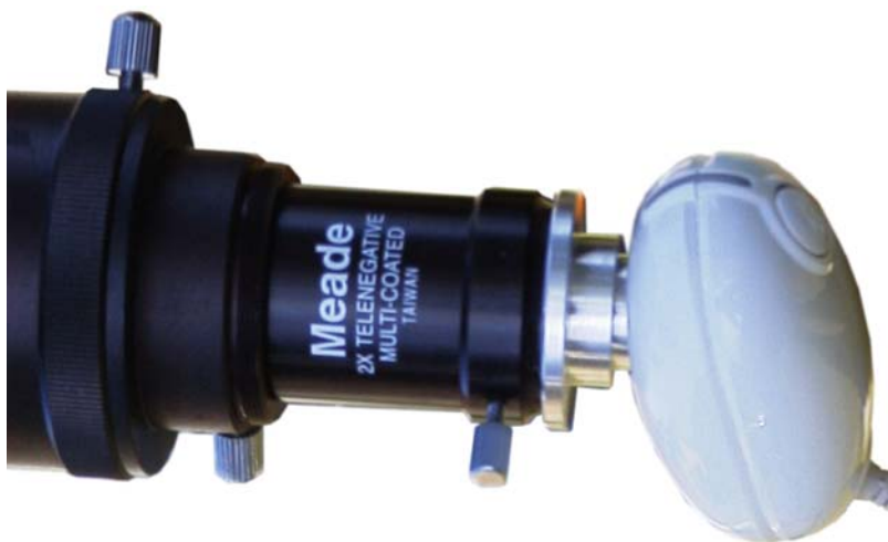
Figure 2.40. Prime focus imaging at the telescope using a Philips ToUcam PCVC740K webcam (photo by Peter Grego).
