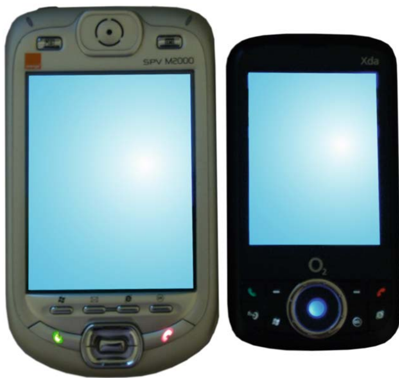
Figure 4.8. The SPV M2000 (3.5-in. diagonal screen) compared with the XDA Orbit (2.8-in. diagonal screen). Cybersketching is easier and more satisfying on the larger screen (photo by Peter Grego).
