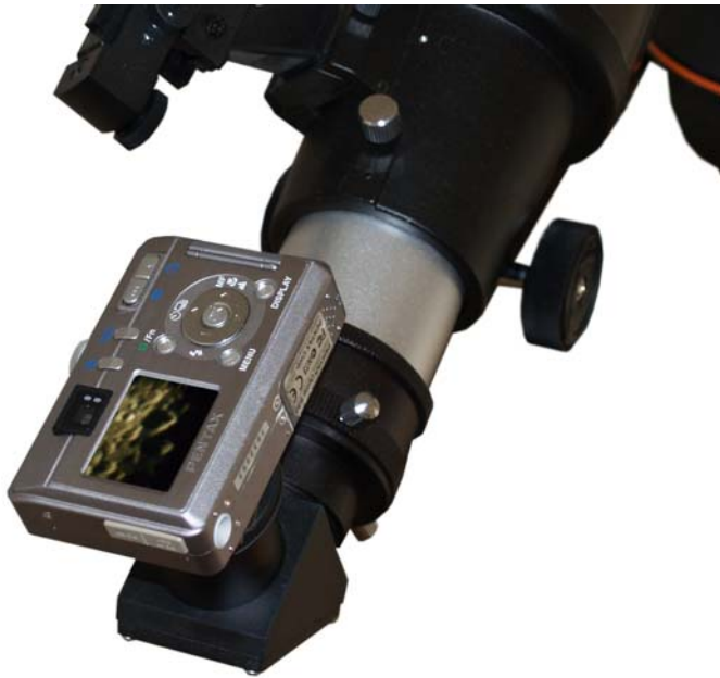
Figure 2.34. The author’s Pentax Optio S30 digicam, set up for afocal imaging through a 100-mm refractor (photo by Peter Grego).
