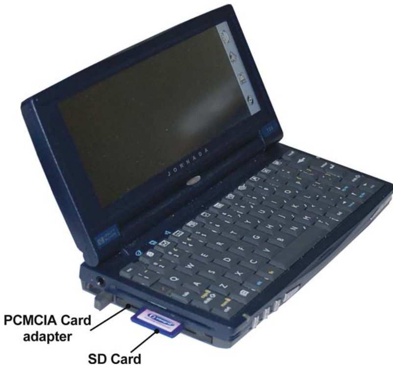
Figure 5.1. The author's Jornada 720 handheld computer, showing the location of the PCMCIA Card adapter (with SD card inserted) – useful for storing and transferring data and graphics files between computers (photo by Peter Grego).
