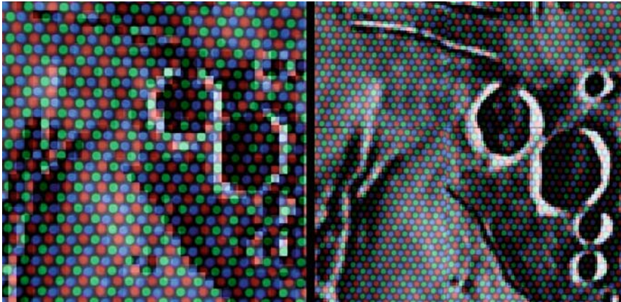
Figure 2.22. Simulation of a low-resolution CRT display ( high dot pitch ) compared with a higher resolution display ( low dot pitch ), both showing the same image and viewed from the same close distance (photo by Peter Grego).
