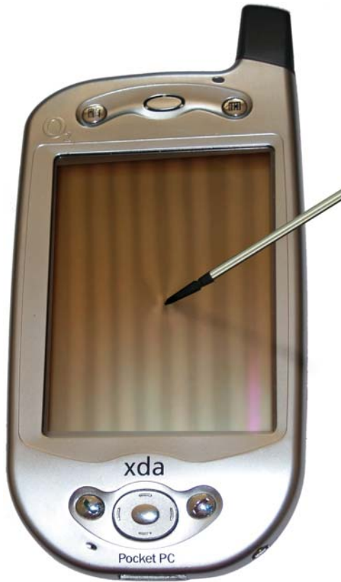
Figure 3.3. The author's XDA, a PDA with a resistive touchscreen. This image shows a simulation of the slight distortion of the upper layer of the screen (power switched off) when pressure is applied with a stylus. If the unit were switched on, the LCD image beneath would appear undistorted, however (photo by Peter Grego).
