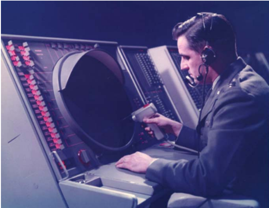
Figure 1.9. SAGE in operation. A USAF radar operator applies a light pen to the screen to bring up information about the displayed target (USAF).
