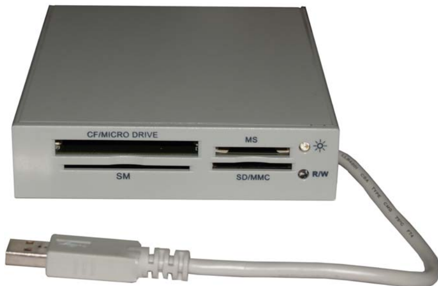
Figure 5.10. A USB flash card reader, capable of reading and writing a variety of memory cards (photo by Peter Grego).
