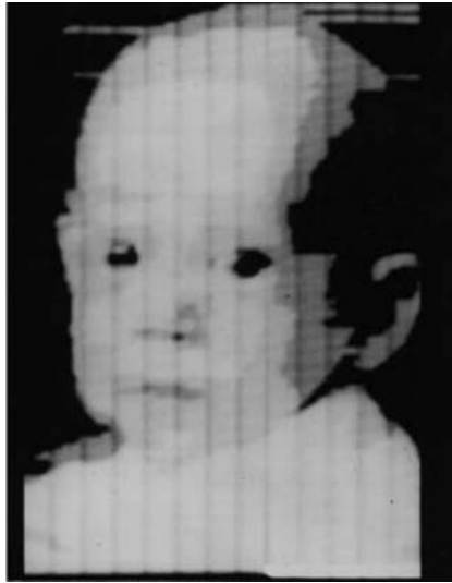
Figure 2.32. This black and white picture of scientist Russell Kirsch's 3-month-old son, Walden, is the first picture ever scanned. It has a resolution of 176 \times 176 pixels (Russell Kirsch, Wikimedia Commons).
