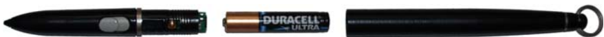
Figure 2.17. The active stylus of the Hammerhead HH3 tough tablet PC, showing the AAAA battery and the internal electronics (photo by Peter Grego).
