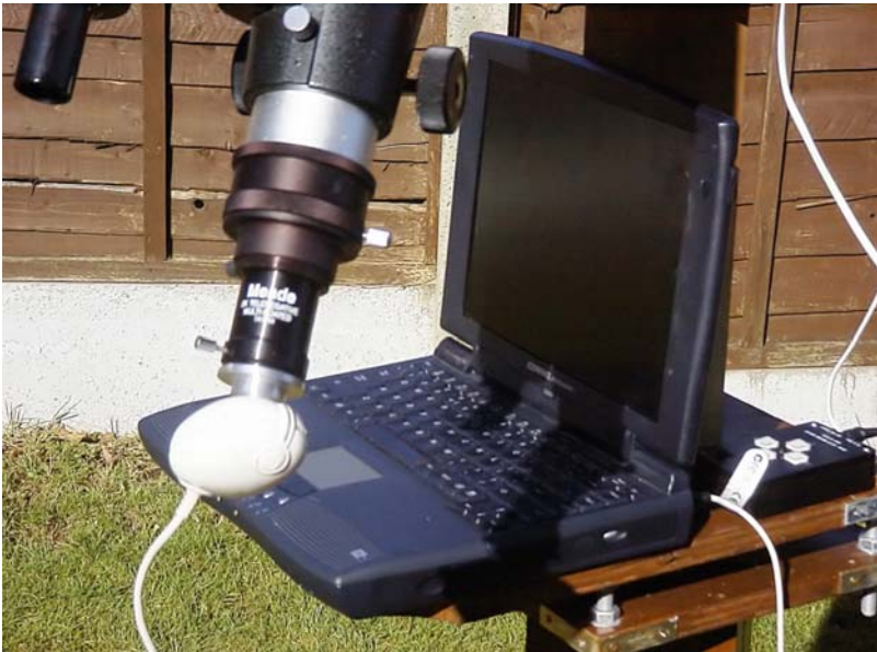
Figure 3.2. The author's vintage Compaq Presario 1200 laptop has an old-style passive matrix display. It is shown here set up for webcam imaging (photo by Peter Grego).
