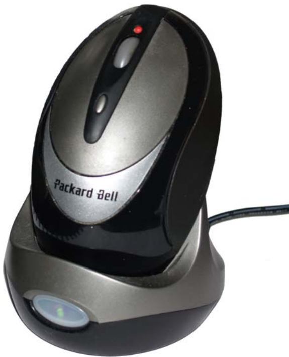
Figure 2.14. The author's main mouse, a Packard Bell PB-EWRO1 cordless rechargeable optical mouse, shown in its cradle (photo by Peter Grego).
