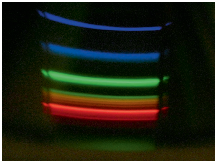
Fig. 5.12. Diffracted light from a low energy domestic bulb.
