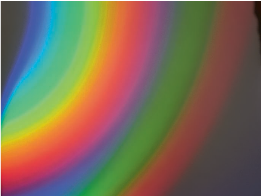
Fig. 5.8. Camera shot of a spectrum of sunlight from a CD.
