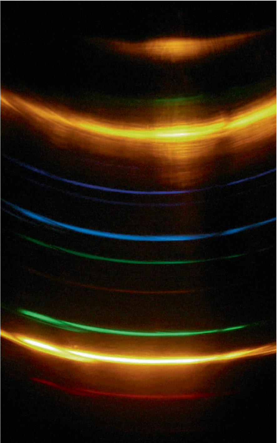
Fig. 5.11. Diffraction spectrum of light from sodium street lamp. Spectral colors characteristic of that particular light source are easily identified.
