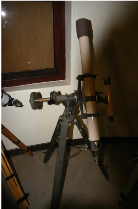
A 3-in. Swift refractor on a sturdy equatorial mount
