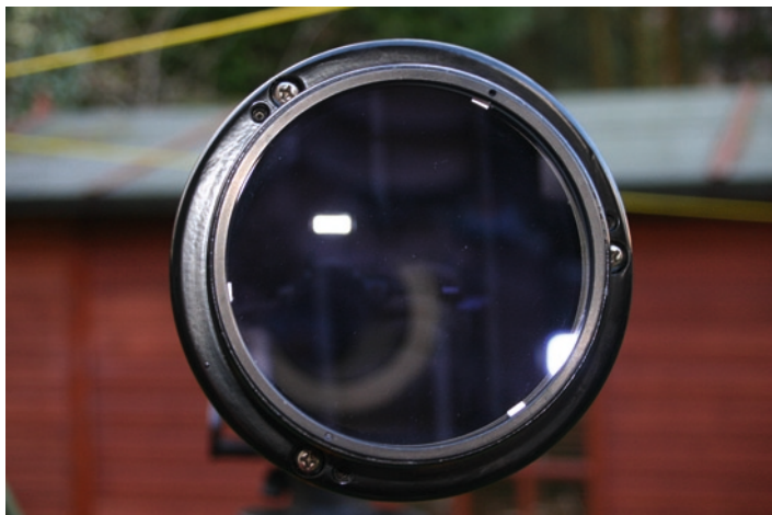
The Fraunhofer achromatic doublet objective of the Skylight F/15 (Image by the author)
