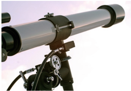
A manually operated equatorial mount carrying a classic Towa 80 mm F/15 refractor (Image credit: Dennis Boon)
