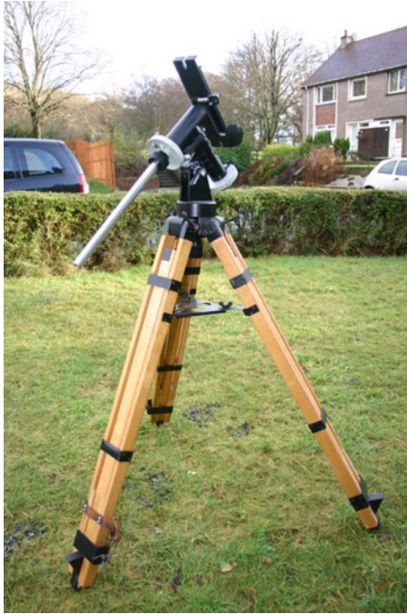
A lightweight German equatorial mount (Image by the author)
