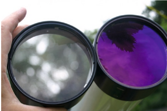
Antireflection coatings can vary dramatically from scope to scope. (Image by the author)
