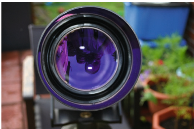
The intense purplish anti-reflection coatings on the Tal 100R objective (Image by the author)
