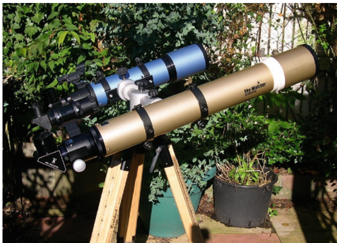
The Sky-Watcher's ED 80 (blue tube) mounted side by side with the ED 100 (Image credit: A. McEwan)
