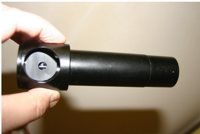
An indispensable collimating tool, the Cheshire eyepiece (Image by the author)
