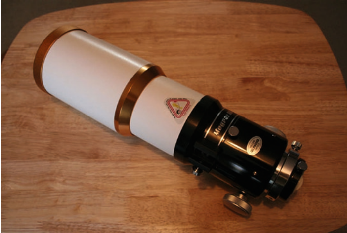
The 80 mm F/6 William Optics/TMB Megrez triplet Apo (Image courtesy: Lee Townend)
