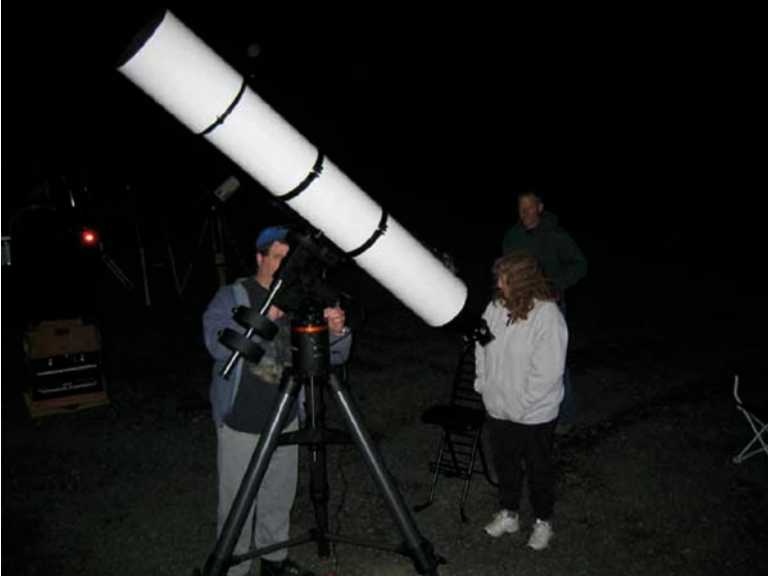
The APM 8-in. F/9 achromat ready for a night under the stars (Image credit: Karl Krasley)
