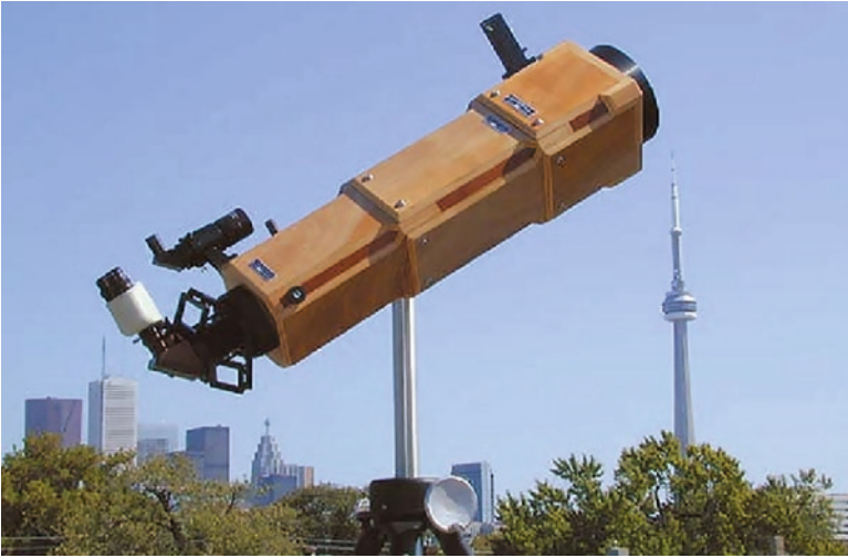
Joseph Drapell's 8-in. F/5 "Travel Star" rich-field achromat with Toronto's CN tower in the foreground (Image credit: Joe Drapell)
