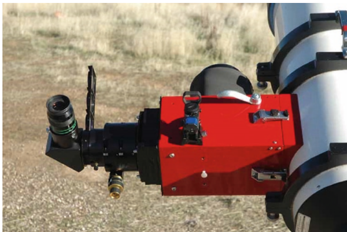
A close up of the focuser on Bob Ayer's 8-in. F/6 refractor with a mated filter slide attached to the diagonal
