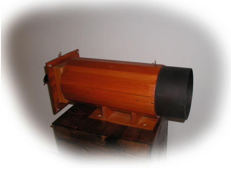
Fig. 4.2 The large copyscope. Note the dowels sticking out of the sides of the cradle at the balance point. They allow mounting on the PVC-concrete mount. You can see the results of drifting the lens apart at the front, to the right of the lens cell. The round item to the left of the telescope is a salvaged piece of tubing that fits the front of the lens cell and serves to protect the front of the lens from stray light
