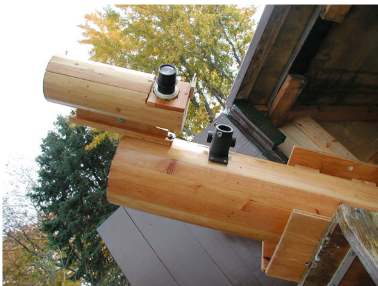
Fig. 8.5 This picture shows the entire mounting and finder attached to the f9 Newtonian
