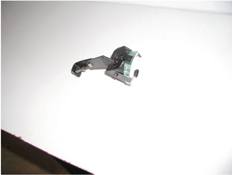
Fig. 6.4 Diagonal mirror held by clips to a wood backing and a single vein spider
