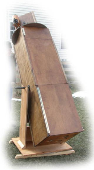
Fig. 10.6 The 12.5-telescope on the dobsonian mount
