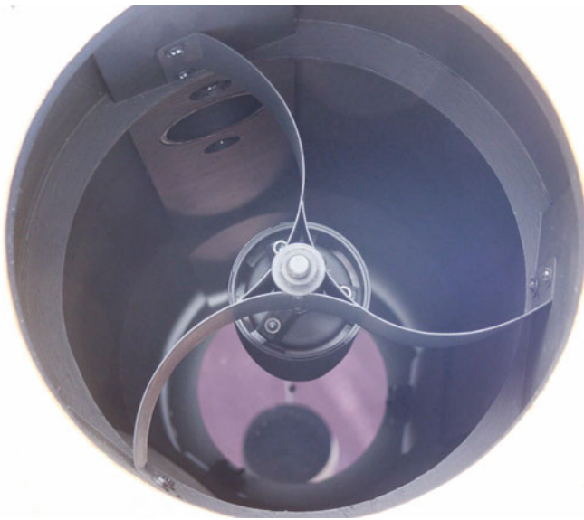
Fig. 6.5 Three-vane spider (Courtesy of Gary Frishkorn, Westminster Astronomical Society)
