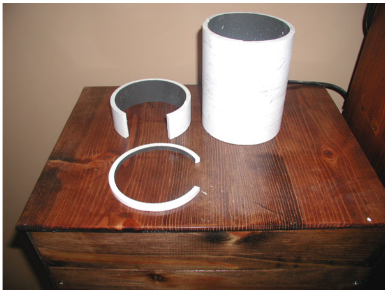
Fig. 13.2 Parts for an Objective cell
