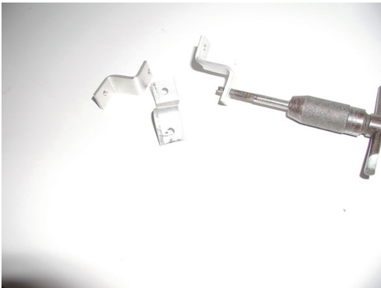
Fig. 6.8 Z collimation clips for a main mirror
