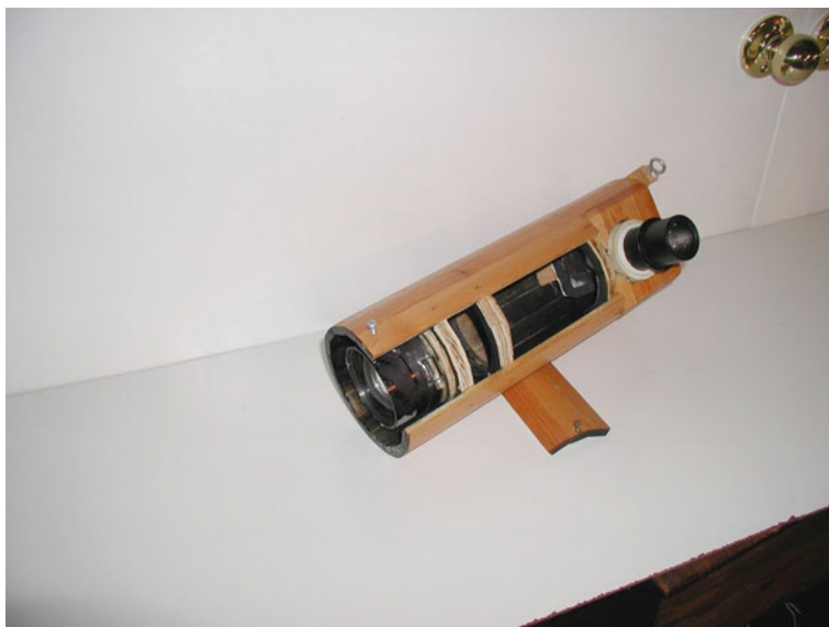
Fig. 8.4 Finder with access plate removed
