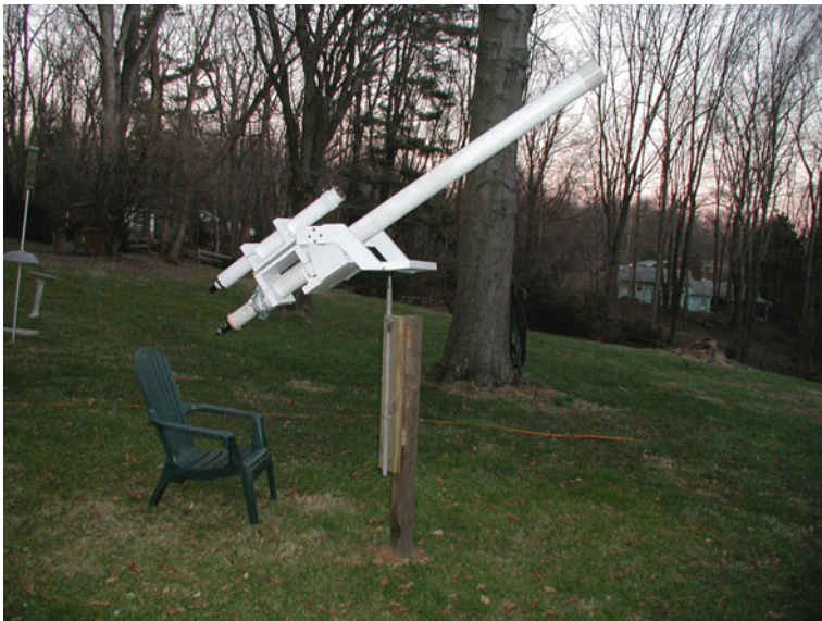
Fig. 7.9 Long focal length refractor in a PVC tube
