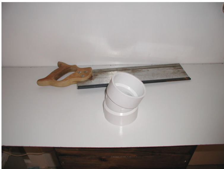
Fig. 13.1 PVC Coupling to be sawed into retaining rings
