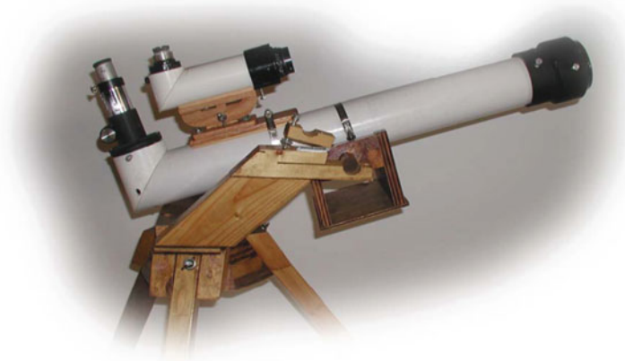
Fig. 5.1 Complete 80 mm telescope
