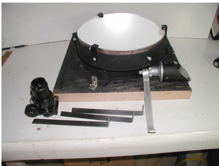
Fig. 10.3 Mirror, cell, baseboard, diagonal, stalk, and stabilizers
