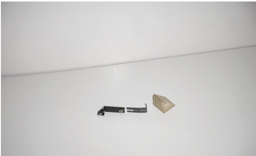
Fig. 6.6 Parts for a single vane spider
