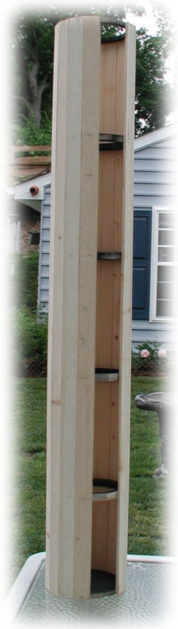
Fig. 9.4 Wooden tube for f9 Newtonian
