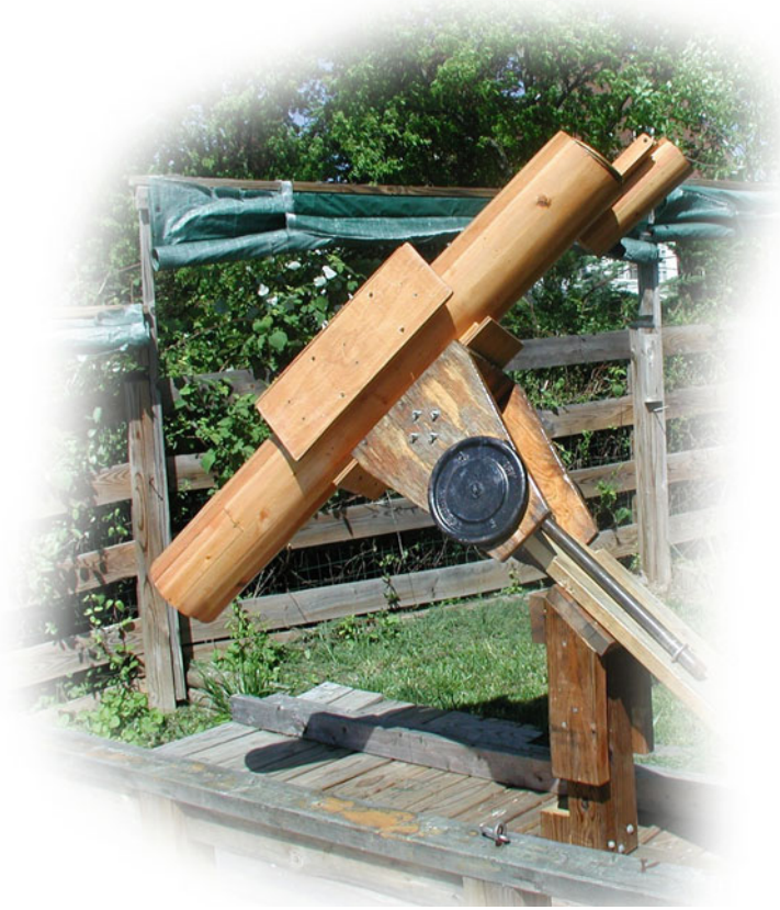
Fig. 11.3 A permanent pipe mounting with the 6-inch long (f9) Newtonian
