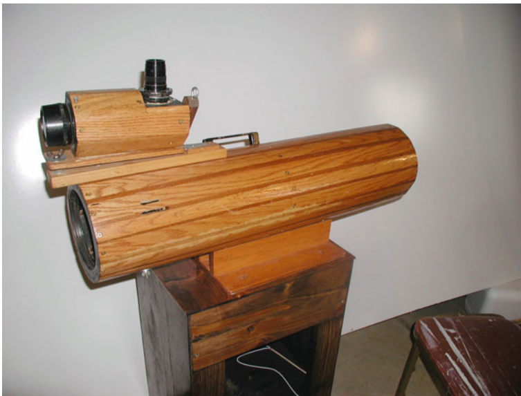
Fig. 6.1 A web-based short Newtonian with a wood tube
