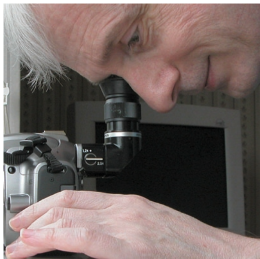
Fig. 11.8. A right angle magnifier fitted over the DSLR viewfinder can make visual focusing easier. Image: Martin Mobberley.
