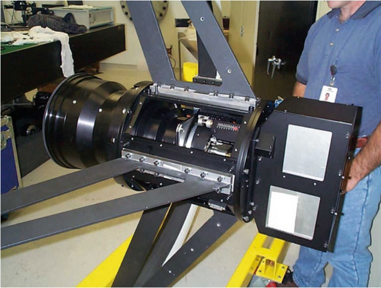
Fig. 3.3. The massive NEAT CCD camera mounted on the secondary mirror support ring of the 1.2 m Maui Space Surveillance Site telescope. Image: Boeing/JPL/NASA.
