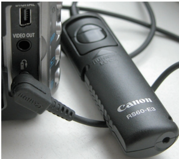
Fig. 11.7. A hands-free remote control for your DSLR will eliminate camera shake from the user’s trigger finger. Image: Martin Mobberley.
