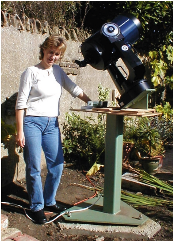
Fig. 11.5. A telescope housing can be simple, but effective. Karen Holland’s 25-cm Schmidt–Cassegrain sits on an elevated pillar and is protected by a lightweight box when not in use. Image: Karen Holland.
