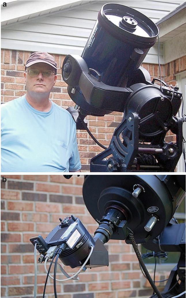
Fig. 15.9. (a) Charles Bell of Vicksburg, Mississippi is one of the world's most active comet imagers. Image: Charles Bell. (b) The business end of Charles Bell's 30-cm Schmidt-Cassegrain incorporates a focal reducer, an SBIG ST-8XME CCD, an SBIG AO-7 adaptive optics guider and an SBIG photometric filter wheel. Image: Charles Bell.
