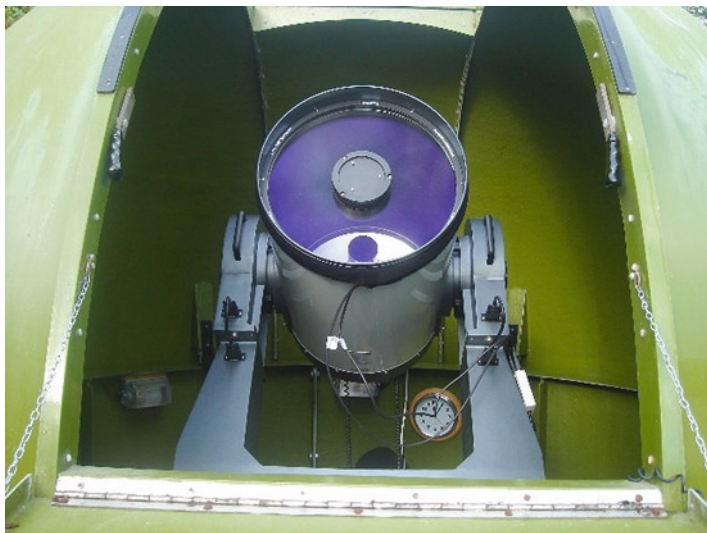
Fig. 9.2. The 0.4-m aperture Schmidt–Cassegrain of NEO chaser extraordinaire Peter Birtwhistle at Great Shefford UK, viewed through the dome slit. Image: Peter Birtwhistle.
