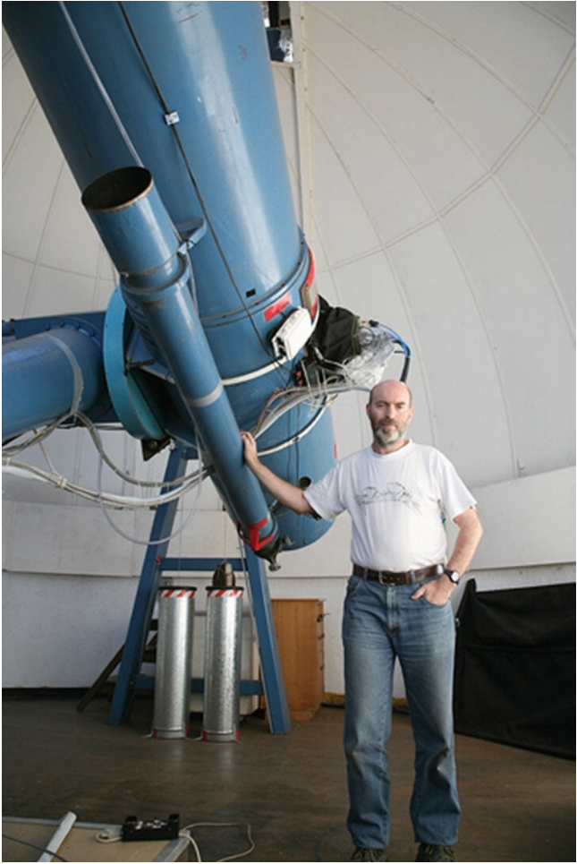
Fig. 3.5. Rob McNaught with the modified 52-cm f/3.4 Uppsala Schmidt telescope. Image: Rob McNaught.
