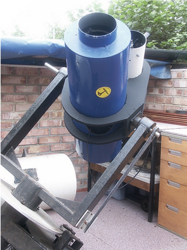
Fig. 12.8. The home made 160 mm f/2.5 Schmidt camera of Mike Harlow, as described in the text. Image: Martin Moberley.
