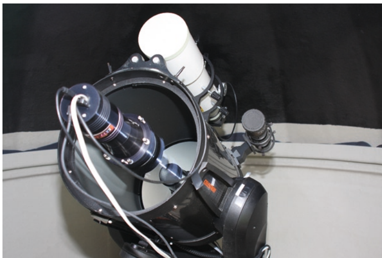
Fig. 12.1. The 11-in. (280-mm) Celestron of Prof. Greg Parker, fitted with a Hyperstar III to give an f/2 system at his New Forest Observatory. A Starlight Xpress SXVF-M25C is attached to the new f/2 focus. This system was used to take the Comet Lulin picture processed by Noel Carboni and shown in Fig. 11.16. Image: Prof. Greg Parker.
