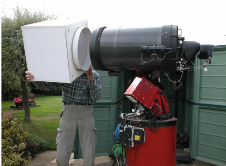
Fig. 11.21. A flat field box can produce an even illumination if a clear twilight sky is not available. Image: Martin Mobberley.
