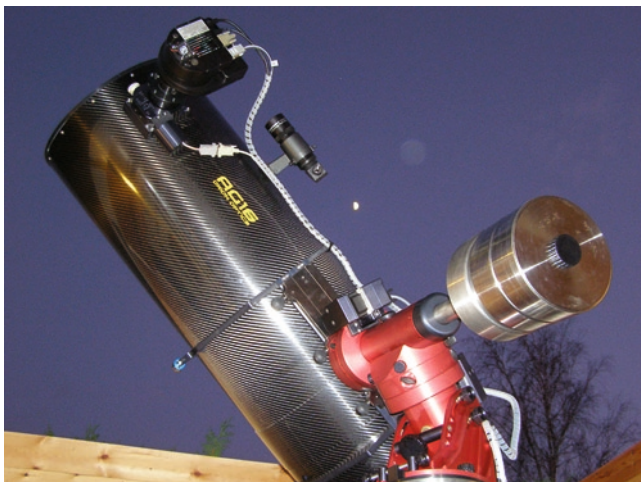
Fig. 15.4. Erik Bryssink's 0.4-m f/3.8 Orion Optics AG16 astrograph mounted on an Italian 10 \mu m GM2000 Qci mount at his run-off roof observatory in Kruikebe, Belgium. Image: Erik Bryssink.
