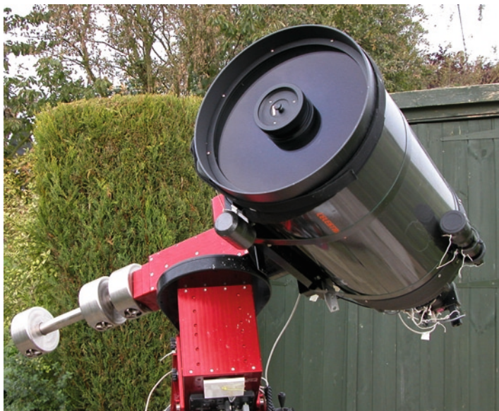
Fig. 11.10. The author's Celestron 14 is mounted on a very high quality Paramount ME equatorial mounting which has a tiny periodic error. Image: Martin Mobberley.
