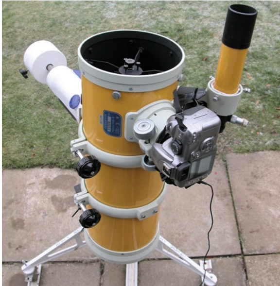
Fig. 12.2. A fast astrograph like Takahashi’s 160-mm aperture f/3.3 Epsilon E-160 is ideal for comets, covering a degree or more of the sky. Image: Martin Mobberley.
