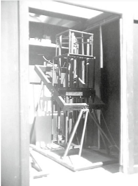
Fig. 4.3. One of Roy Tucker's unusual trio of 35-cm Newtonians which scan the sky using the drift scan technique: the telescopes do not track the stars as the image is downloaded at the rate the sky drifts over the CCD sensor.
