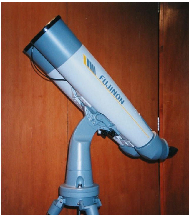
Fig. 4.5. Fujinon’s classic 25×150 binoculars have always been especially popular amongst Japanese comet hunters. Image: Martin Mobberley.
