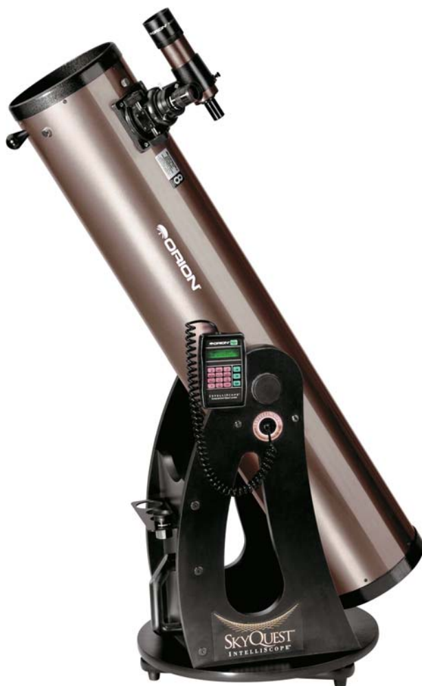
Figure 5.4. Orion's line of SkyQuest IntelliScope Dobsonian reflectors feature Push-Pull-To computerized technology to locate objects. The hand controller (seen here on the 8-inch model) indicates the location of a desired object while the observer moves the telescope until a "null" reading appears on the LCD display. Courtesy of Orion Telescopes & Binoculars.
