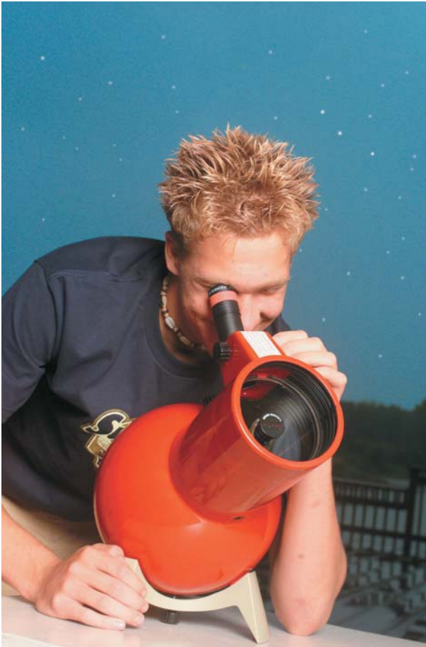
Figure 5.5. The 4.25-inch aperture Edmund Scientifics Astroscan is one of the best-selling small reflectors ever made and it remains one of the most popular RFTs (richest-field-telescope) on the market today. It's 16x eyepiece provides a wide 3-degree field of view (or 6 full-Moon diameters of sky), and its unique optical window protects the system from dust as well as supports its diagonal mirror. Courtesy of Edmund Scientifics.
