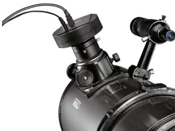
Figure 7.10. Shown here is a CCD color imaging camera attached to the focuser of a Newtonian reflector. This one is intended primarily for use on deep-sky objects, while other models are available for imaging solar system targets such as the Moon and planets. In either case, the output is fed into a PC for viewing and processing. These state-of-the-art devices make it possible for amateur astronomers to routinely take pictures rivaling those of professional observatories! Courtesy of Orion telescopes & Binoculars.
