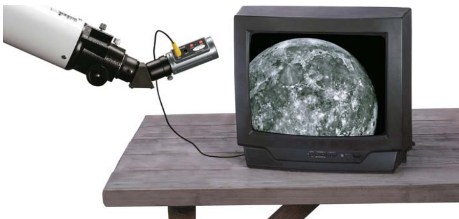
Figure 7.9. Electronic eyepiece cameras (both black & white, and color) like that seen here make video imaging easy and affordable today. The camera output can be displayed in real time on a monitor, or recorded on a VCR or camcorder for viewing later. Courtesy of Orion Telescopes & Binoculars.
