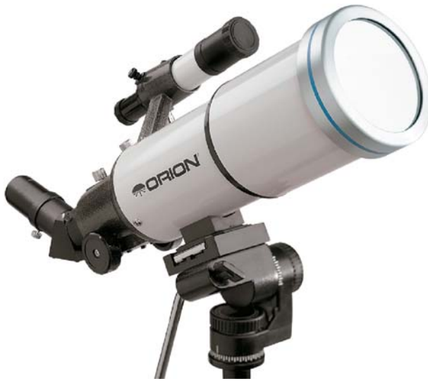
Figure 11.1. A full-aperture optical-glass solar filter mounted over the objective of an 80-mm refractor. (Note the capped finder – a very vital precaution!) While more expensive than Mylar ® solar filters, these provide better image contrast and a more natural-looking yellowish-orange Sun rather than a blue one. Securely mounted, such full-aperture devices are completely safe for viewing our Daytime Star – in contrast to the highly dangerous practice of placing a filter over the eyepiece itself. Courtesy of Orion Telescopes & Binoculars.
