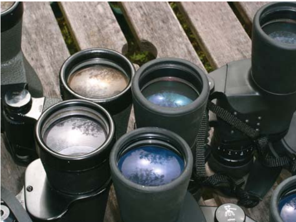
Figure 2.19. Optical coatings. Clockwise from top left: single-layer coated, broadband multicoated, multicoated, uncoated.
