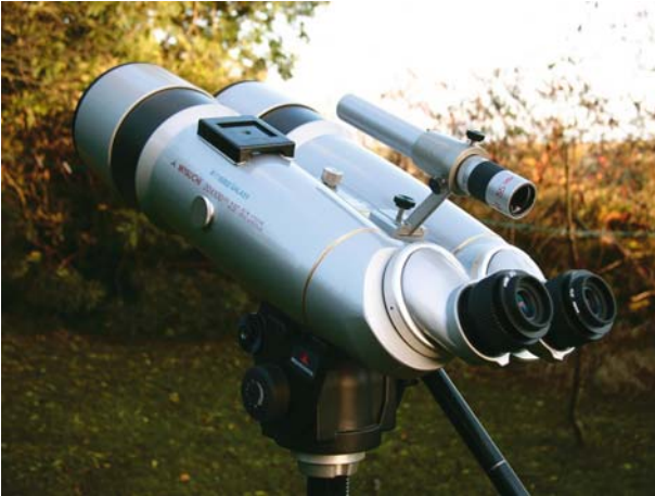
Figure 7.2. 3×12 finder scope with 55-mm eye relief.
