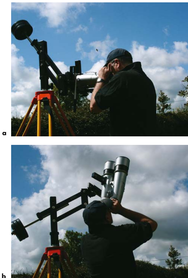
Figure 6.13A,B. A well-designed parallelogram mount allows more than a quarter of the sky to be observed without the observer having to move.
