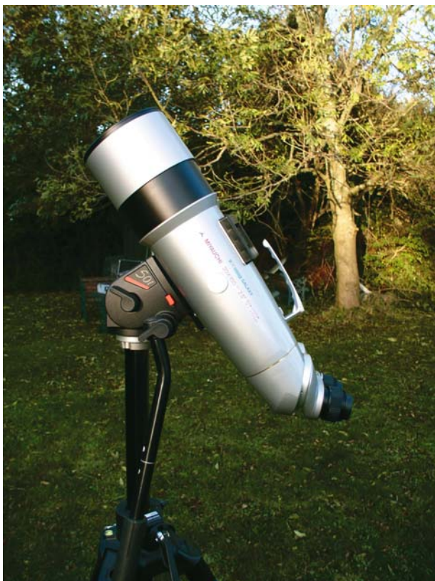
Figure 6.10. With the video head the right way around, the zenith is inaccessible.
