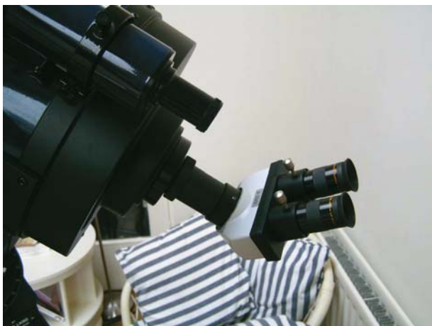
Figure 3.10. Celestron binoviewer attached to a Meade 10" LX50. (Photo: courtesy of Gordon Nason)
