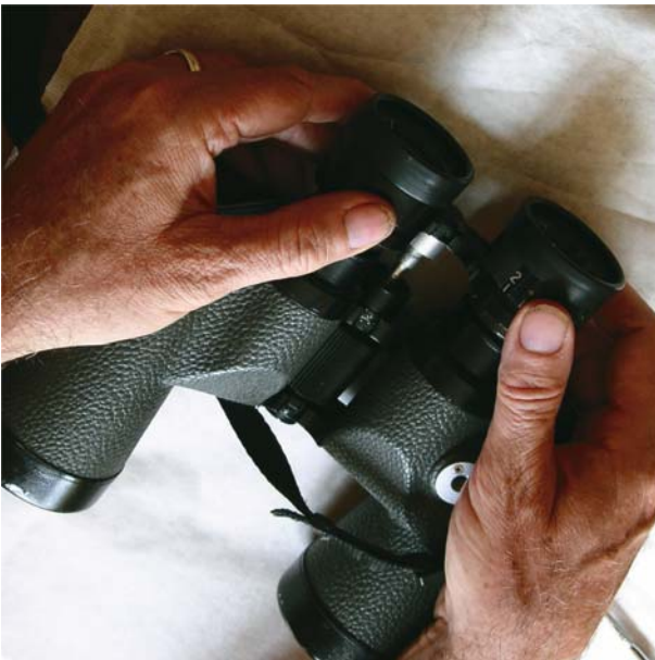
Figure 5.6. The bridge and eyepieces are lifted clear.
