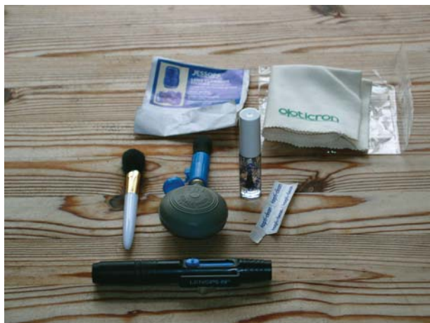
Figure 5.2. Cleaning kit. Top L to R: Lens tissue, microfiber cloth. Middle: camel-hair brush, blower brush, Opti-Clean. Bottom: Lens Pen.
