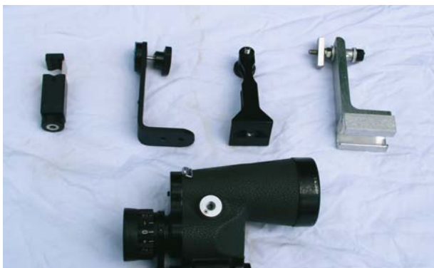
Figure 6.5. Various mounting brackets. Top, L-R: Hinge clamp, Universal L-bracket, roof prism L-bracket, Proprietary (Universal Astronomics) L-bracket. Bottom: Bush in prism housing.
