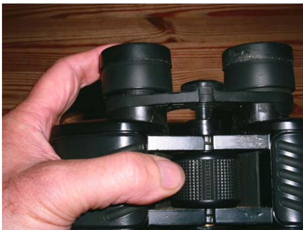
Figure 2.27. The bridge rocks on this center-focus Porro prism binocular.
