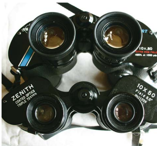
Figure 4.1. Wide-angle eyepieces (top) are of large diameter and may be unusable for people with narrow-set eyes or wide noses.
