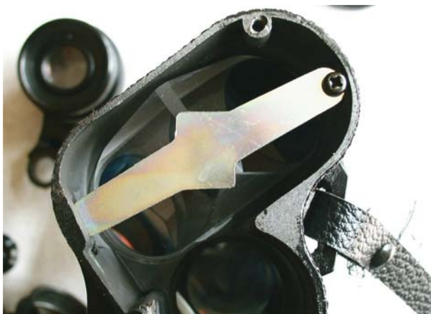
Figure 5.9. Clamped prism in Zeiss-type binoculars.
