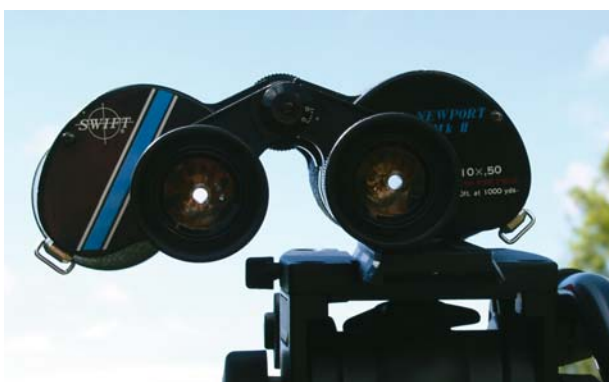
Figure 6.6. Direct mounting bush.
