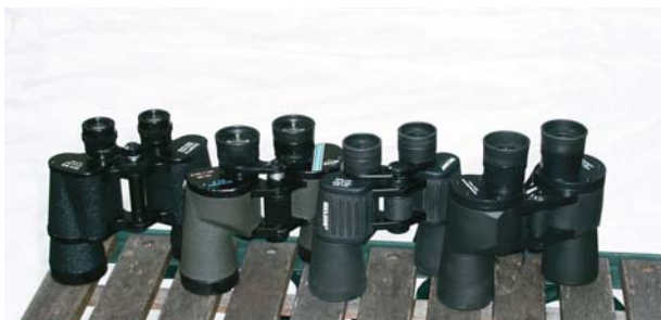
Figure 3.2. Variety of 10×50 porro-prism binoculars. L to R: Older style center-focus Z-body with fixed eyecups (Zenith); Robust center-focus B-body style (Swift Newport); Modern lightweight center-focus Z-body with folding eyecups (Helios Naturesport); Robust individual focus Z-body (Strathspey Marine).
