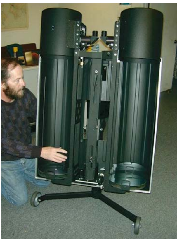
Figure 3.6. 250 mm (10 inch) aperture binocular telescope by JMI. The picture shows the inside of the optical tubes. (Photo: Jim’s Mobile Inc.)
