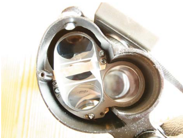
Figure 5.10. Prism cluster in situ.
