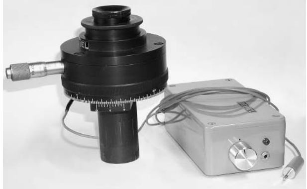
Figure 21.2. The RETEL micrometer and its illumination power supply. (R. Sword (IOA)).
