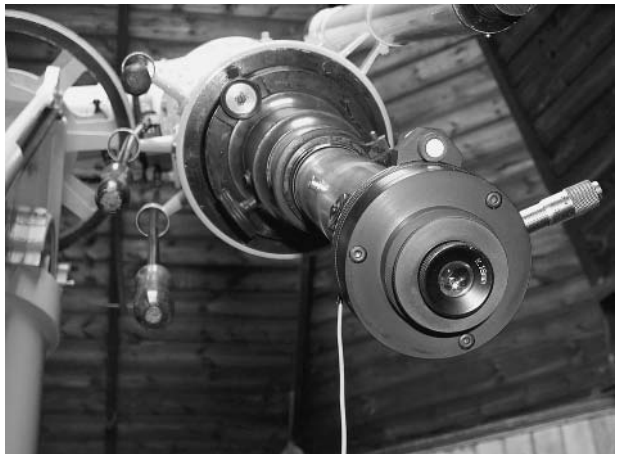
Figure 21.3. The RETEL micrometer and Barlow lens mounted on the 8-inch Thorrowgood refractor. (R. Sword (IOA)).
