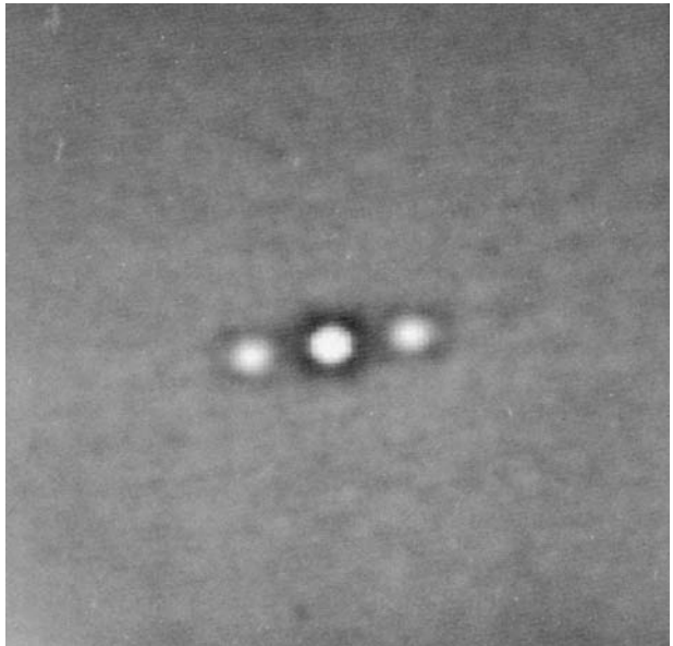
Figure 17.3. A background subtracted autocorrelogram of the binary star \kappa UMa. Adapted from McAlister et al. 1 Printed by kind permission of the American Astronomical Society
