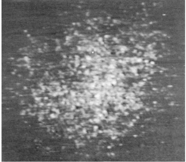
Figure 17.1. A single speckle frame of the star \kappa UMa on the KPNO 4-m. Adapted from McAlister et. al. 1 Printed by kind permission of the American Astronomical Society
