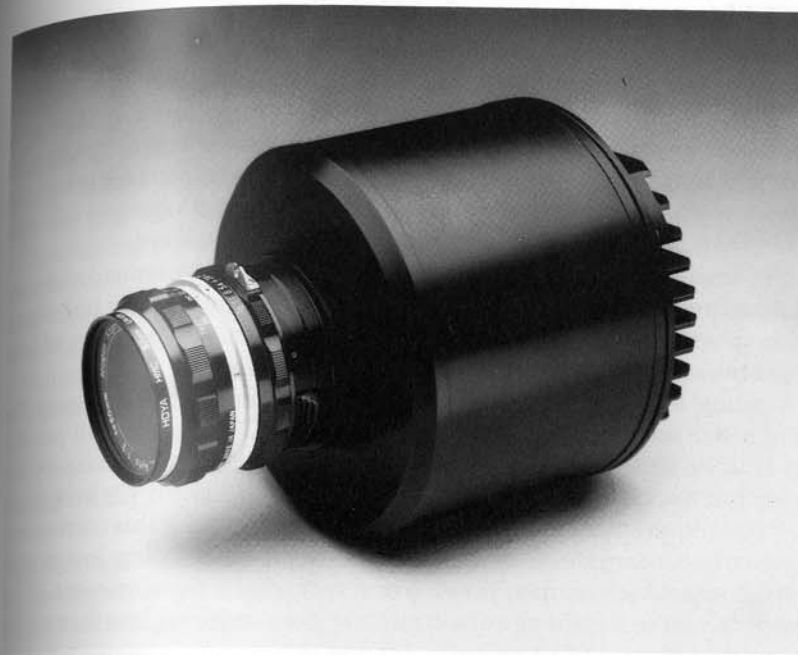
Fig. 15.9 Charge coupled device (CCD) for use with the LyNXX series of planetary and lunar imaging systems. Format: 11024 \times 1024 pixels, pixel size 12 \times 12 micrometres, active area 0.48 \times 0.48 inches ( 1.2 \times 1.2 centimetres), efficiency QE > 50\% at 50 nanometres, charge transfer efficiency 99.998%. (Courtesy of Spectra Source Instruments.)
