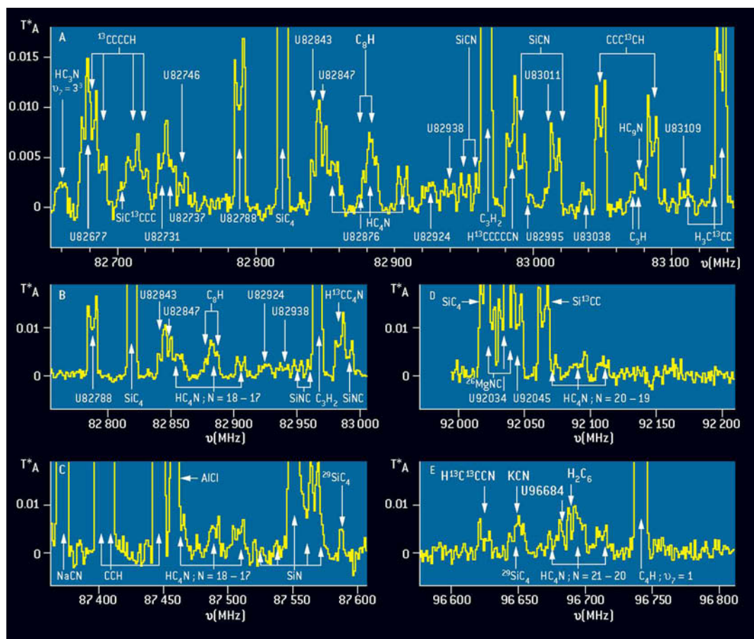
Complex interstellar molecules. Observations (in the millimetric domain) of interstellar clouds or, in these cases, stellar envelopes, reveal the presence of many complex molecules. The letter U refers to unidentified molecules. (After Cernicharo, Ap. J. , 615 , L145 (2004).)
