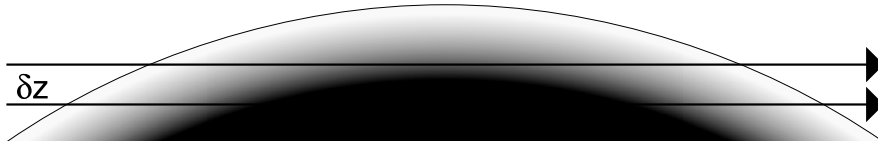
Fig. 38. Two rays separated by \delta z passing tangentially through a planetary atmosphere with scale height H . The opacity along the higher ray is approximately \exp(-\delta z/H) smaller than along the lower ray
