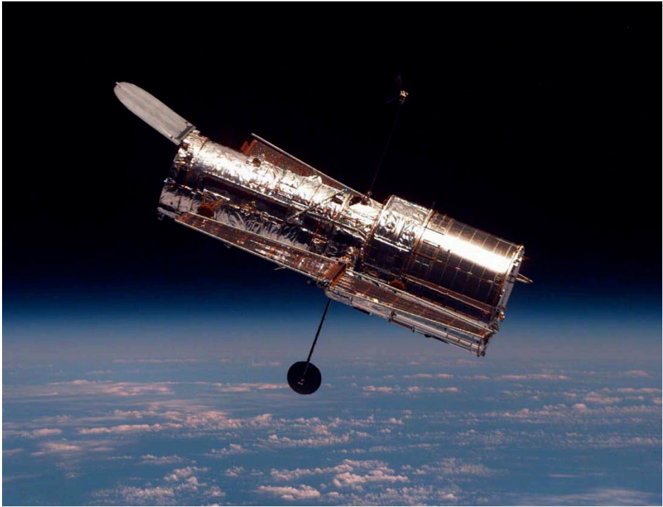
FIGURE 8.8 NASA's Hubble Space Telescope, launched in 1990, and now showing signs of old age. Unless its orbit is boosted it will re-enter the Earth's atmosphere in 2010 or soon after. It has a 2.4 meter diameter mirror. (NASA)
