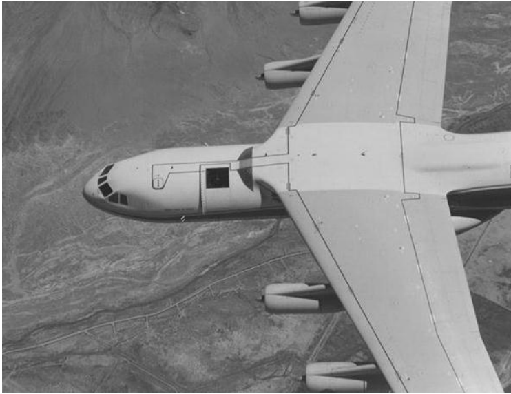
Figure 3.1. The Kuiper Airborne Observatory in flight. Notice the telescope opening in the fuselage just aft of the cockpit. The KAO was decommissioned in 1995.
