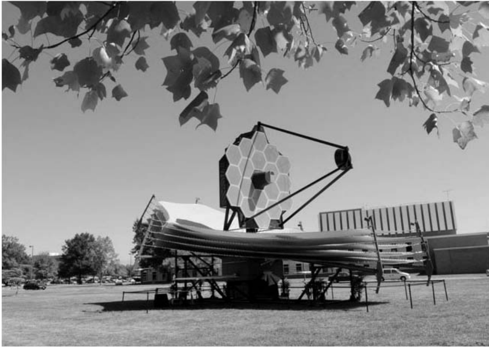
Figure 12.3. A mock-up of the James Webb Space Telescope (JWST), scheduled for launch no earlier than 2013, is on display at NASA's Goddard Space Flight Center in Greenbelt, Maryland. JWST is a more capable version of the Hubble Space Telescope and will orbit the Sun in Earth's L2 Lagrangian point.
