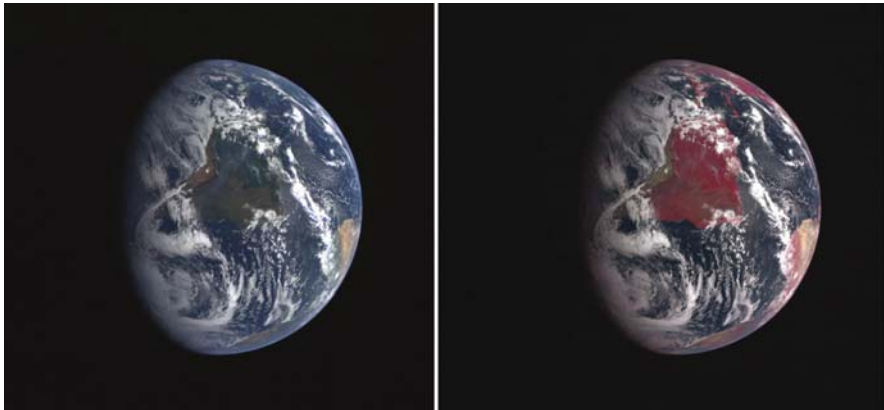
Fig. 1.21 Earth images taken by the wide-angle camera of MESSENGER at 102,000 km above the Earth. ( Left ) Composite made from combining filters with peak sensitivities at 480, 560 and 630 nm (B, G and R filters, respectively). ( Right ) Composite made from combining the filters at 560, 630 and 750 nm. Credit: NASA/Johns Hopkins University Applied Physics Laboratory/Carnegie Institution of Washington. Image PIA10122 of the Planetary Photojournal
