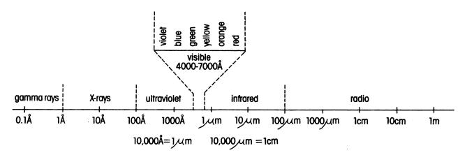
Schematic diagram of the electromagnetic spectrum, ranging from the shortest wavelengths (gamma rays) to the longest (radio waves). The wavelength of light is measured in Ångstroms (Å), micrometers ( $\Box$ m), centimeters (cm) and meters (m).
