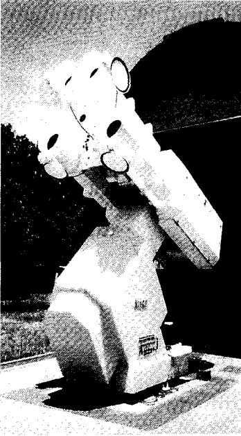
Figure 2.15 Solar flare telescope consisting of 4 telescopes at the NAOJ.
