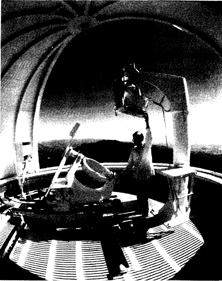
Figure 7.2 (b) The 60-cm 2-mirror coelostat of Mount Wilson observatory. Observer Pam Gilman adjusts the 2 nd flat mirror to direct the sunlight to a 30-cm objective triplet lens, forming a 38-cm diameter solar image at the base of the tower in the observing room.
