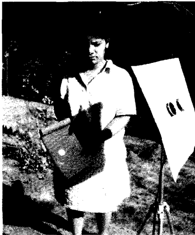
Figure 7.1 Simple and safe method to examine the solar image is by projecting the image on a white card. The image is formed by a small 50-150 mm aperture size refracting telescope with an eyepiece, or even by a binocular.
