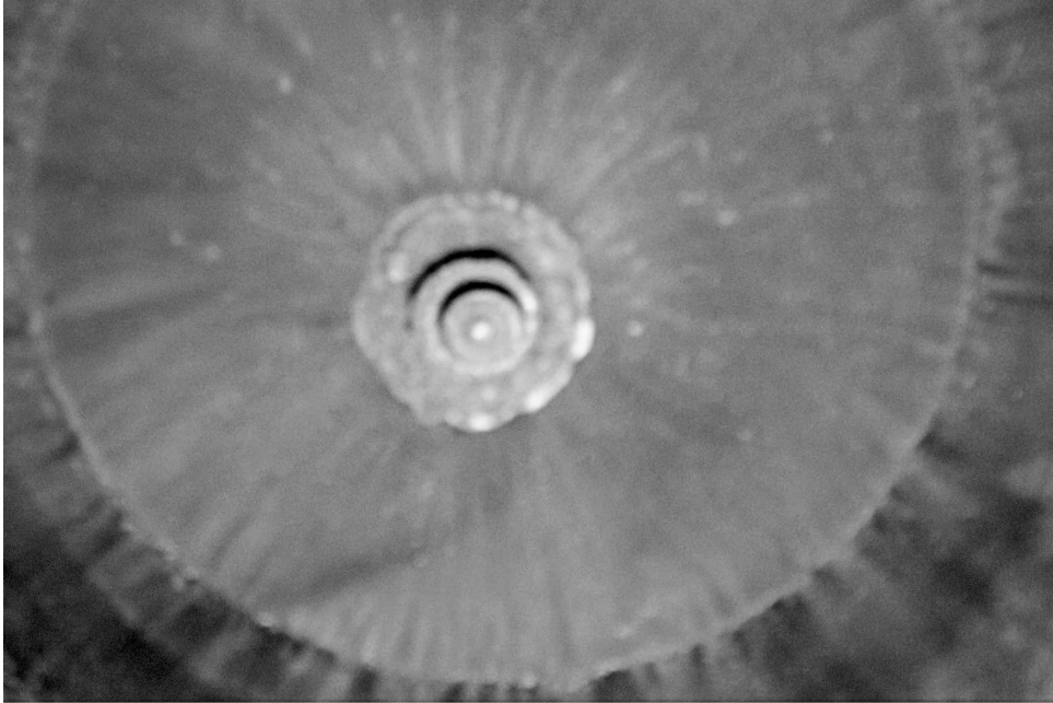
Figure 11.5 Craters from tests. Notice the tiers of crater diameter corresponding to the tests performed at different explosive depths. (The outer ring nearly spanning the photograph demarcates the inner diameter of the steel pipe used to protect the wiring.)
