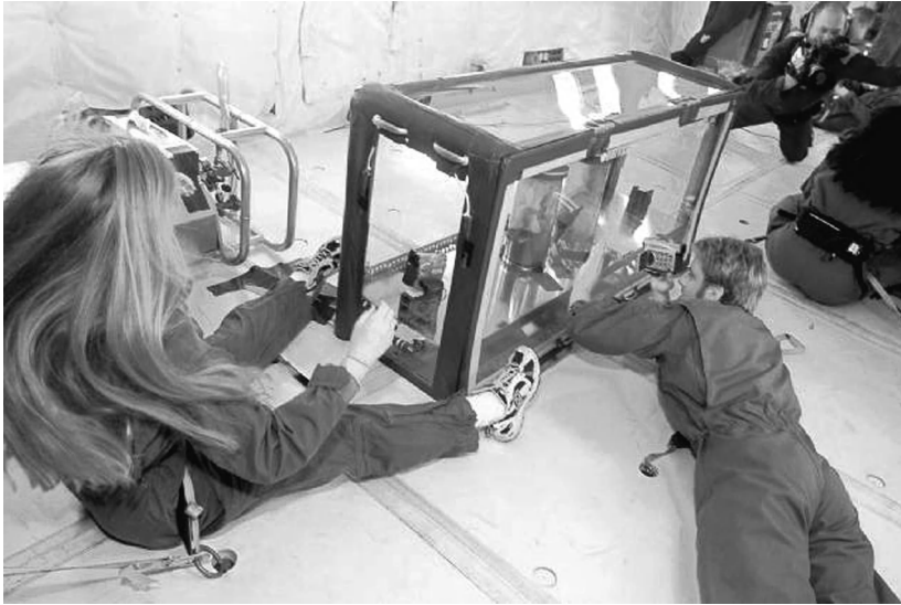
Figure 15.8 Undergraduate students Amber Holley and Mike Meyer operating the apparatus for campaign II. The apparatus consists of two 15-cm Plexiglas cylinders containing sand and iron filings with similar grain sizes and in similar proportions to those of chondritic meteorites. The experimenters recorded the behavior of the beds using digital cameras as the KC-135 went through nearly 80 parabolas of positive gravity, microgravity, and negative gravity and then positive gravity again.
