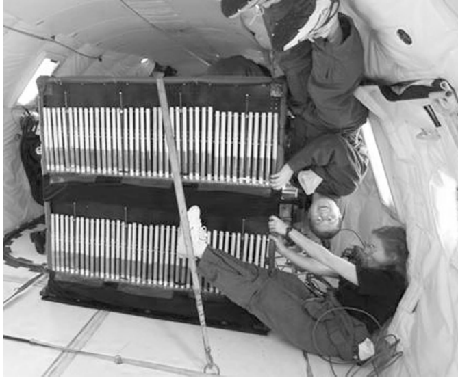
Figure 15.6 Undergraduate students Ryan Godsey and Katrina Bogdon with the apparatus for campaign I. The apparatus consists of 310 2.5-cm Plexiglas tubes containing sand and iron files of chondritic grain sizes and in various proportions. The white “pistons” were depressed while the beds were under microgravity conditions in order to “freeze-in” any segregation that may have occurred during flight.
