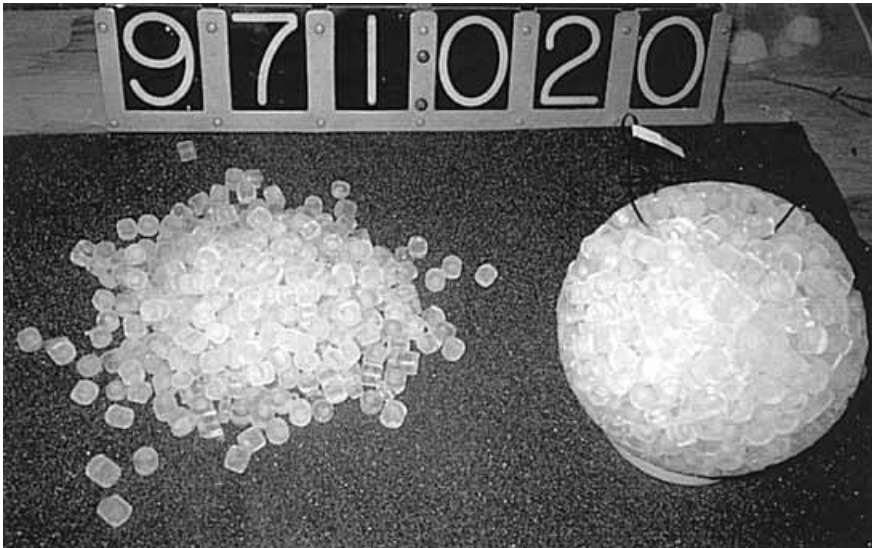
Figure 9.2 A test target representing a planetesimal in the trans-Neptunian region. It was assembled from a bag of commercially available ice cubes. (Eileen Ryan.)
