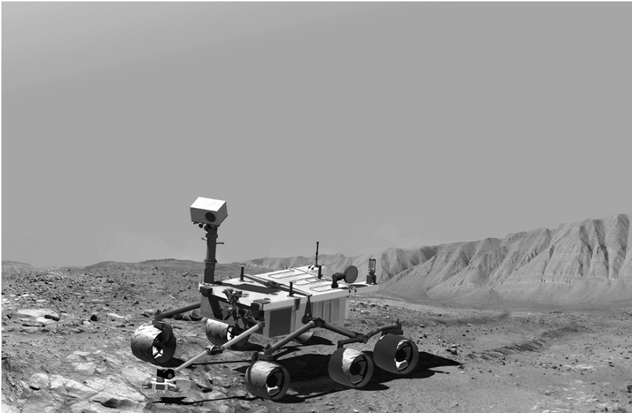
Figure 102: Artist's impression of NASA/JPL Mars Science Laboratory (MSL). MSL will be larger than the MER rovers, be able to travel over 10 kilometers from its landing site, and look for evidence of biology on Mars. [Credit: NASA/JPL]
