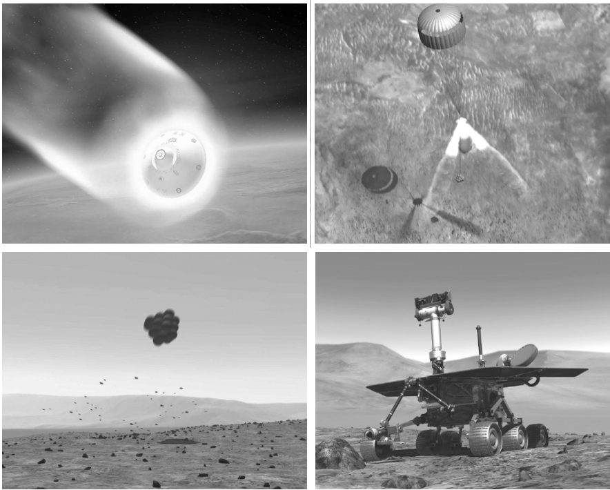
Figure 75: A Mars Exploration Rover (MER) enters the Martian atmosphere. With the parachute deployed the retrorockets fire, suspending the lander at 12 meters from the surface. Protected by airbags, the lander is dropped and bounces along the surface. The lander's petals then unfold and the rover egresses. [Credit: NASA/JPL]
