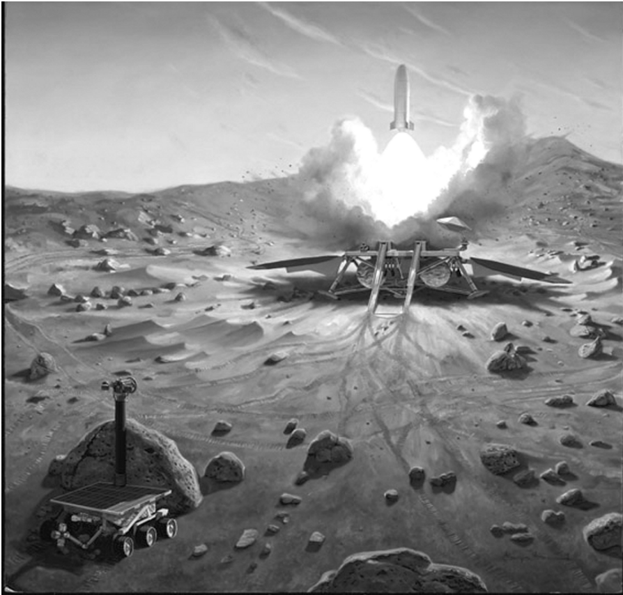
Figure 106: Artist's impression of the launch of a Mars Ascent Vehicle (MAV), bringing samples into Mars orbit where they will be collected and returned to Earth. It is likely that such a mission will take place in the latter half of the next decade. [Credit: NASA/JPL]
