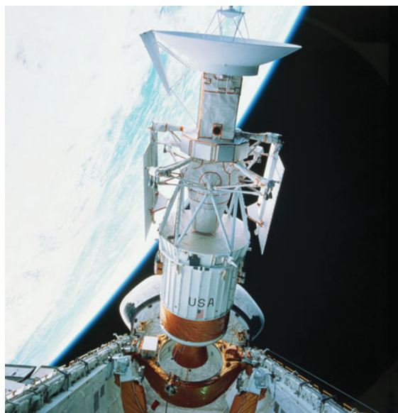
The Magellan spacecraft and an attached rocket are released into a temporary orbit around Earth from the payload bay of the space shuttle Atlantis in 1989. Shortly afterward, the rocket propelled Magellan on a course that took it around the sun and then into orbit around Venus.
