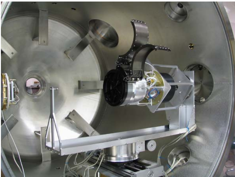
Fig. 27 SWAP instrument mounted on four-axis positioning system
