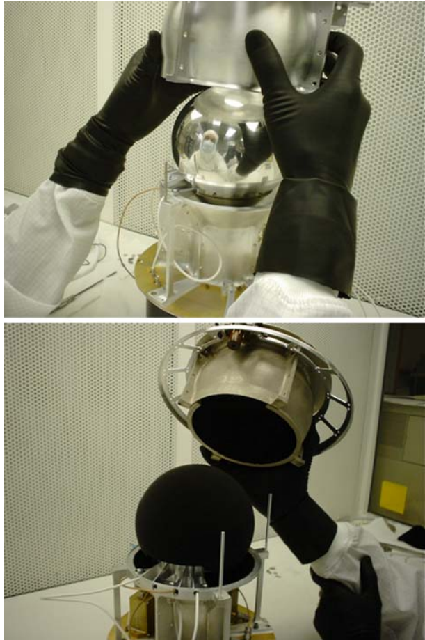
Fig. 14 Cantilevered inner-ESA dome with ( bottom panel ) and without ( top panel ) blackening
