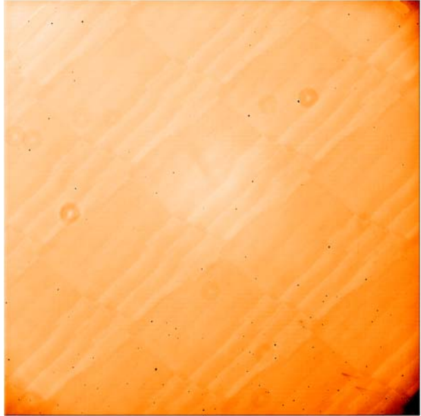
Fig. 8 Provisional flat-field measured at APL: logarithmic stretch from 0.95 ( black ) to 1.05 ( white ). Dust particles form “donuts” and dark spots. There is 4% vignetting in the corners , but in the upper left corner and in the center of the field , there is excess brightness from image ghosting which is not removed in preliminary processing
