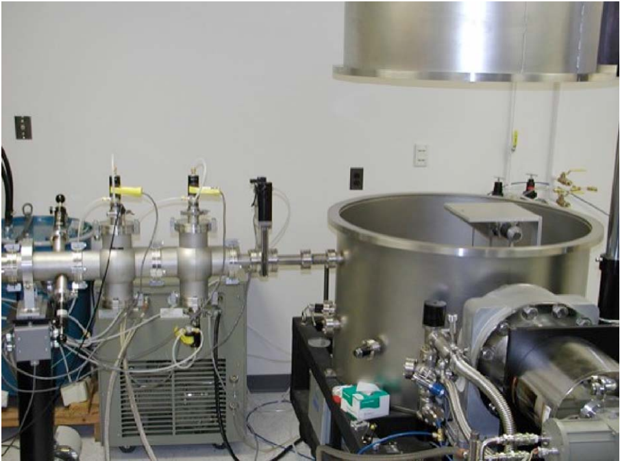
Fig. 19 The vacuum chamber used in calibrating the PEPSSI unit. The beam line enters the chamber horizontally from left to right in the picture
