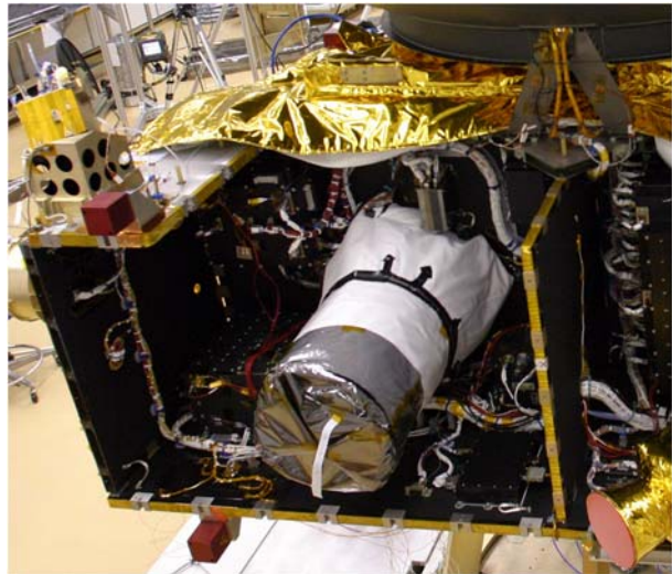
Fig. 2 LORRI mounted within New Horizons spacecraft, with outer panels of spacecraft removed. LORRI is wrapped in thermal blanketing, cover door closed
