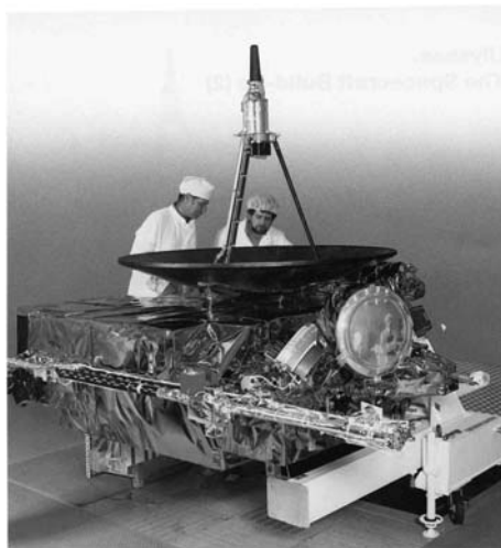
Figure 7.6 The spacecraft Ulysses before launch, covered with a conductive coating. (Photograph by Dornier GmbH.)
