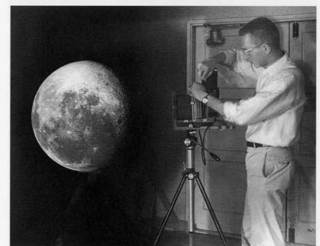
Bill Hartmann photographing telescopic images of the Moon projected onto a large white hemisphere.
