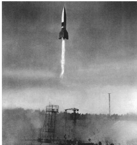
Figure 2.1 The V-2 Ballistic Missile of World War II [Deutsches Museum] The V-2 was the first vehicle to reach space height, and was the progenitor of all subsequent ballistic missiles and launch vehicles.
