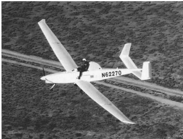
Figure 12.3 Raptor Experimental Unmanned Aeroplane with Safety Pilot [Scaled Composites] Safety pilots are sometimes used to reduce the risk, and hence the overall cost, of the early flights of unmanned aeroplanes. They can take over if the computer is set incorrectly or fails. Likewise, pilots could reduce the risk and cost of spaceplane flights.
