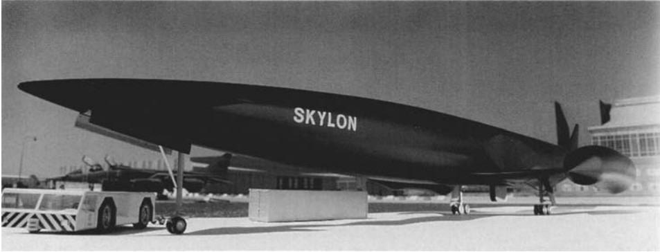
Figure 8.8 The Proposed SKYLON Single Stage to Orbit Spaceplane [Reaction Engines] Skylon uses a combined air-breathing and rocket engine to reduce the propellant mass fraction needed to reach orbit with a single stage spaceplane.
