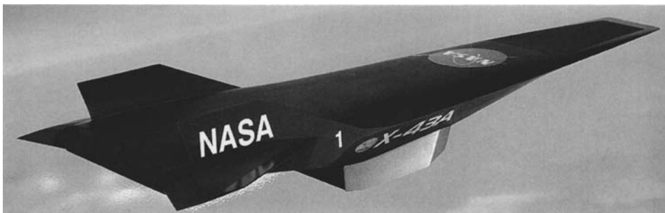
Figure 8.9 The X-43 Scramjet Research Vehicle [NASA] The 3.7 metres long X-43 is designed to test supersonic combustion ramjets in flight. These offer the long-term prospect of an aeroplane-like single stage to orbit vehicle.
