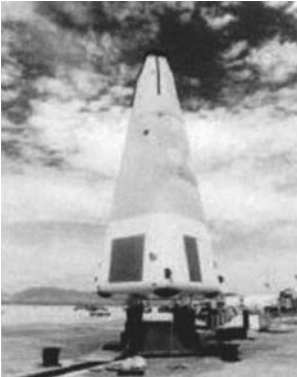
The DC-X demonstrator for a vertical take-off, vertical landing reusable launcher made 12 flights from 1993 to 1996. It cost about $120 million.
