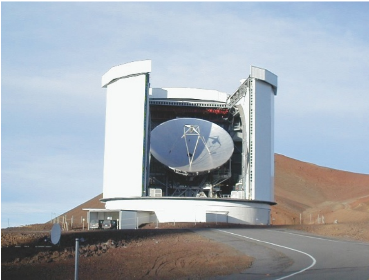
Fig. 1.23. The JCMT has a 15-m dish. It is protected by the largest single piece of Gore-Tex, which has a transmissivity of 97% at submillimeter wavelengths
