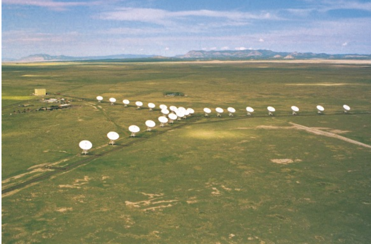
Fig. 1.21. The Very Large Array (VLA) in New Mexico consists of 27 antennae with a diameter of 25 m each that can be moved on rails. It is used in four different configurations that vary in the separation of the telescopes; switching configurations takes about two weeks
