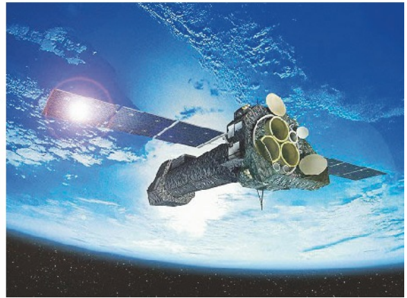
liptical orbit permits long uninterrupted exposures. Lower right: XMM-Newton was launched in December 1999 and is planned to be used for 10 years. Observations are carried out with three telescopes at energies between 0.1 and 15 keV
