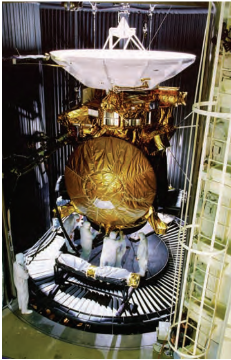
The Cassini probe undergoes thermal testing at the Jet Propulsion Laboratory in Pasadena, California. (NASA)
