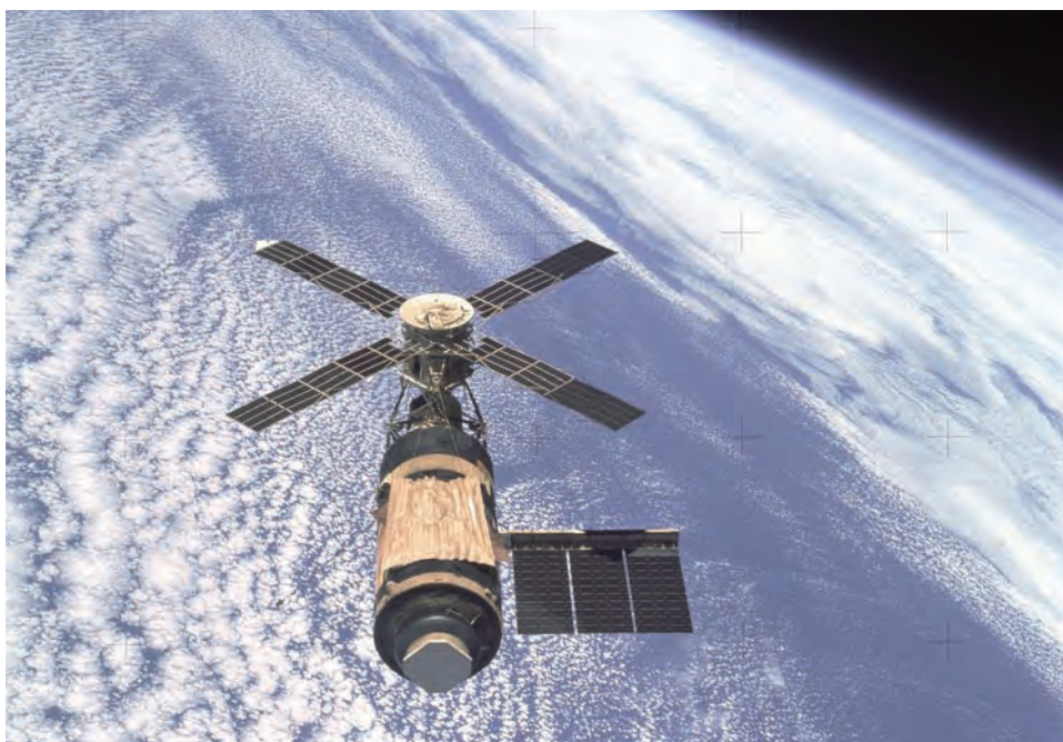
Skylab was the first U.S. space station and had a highly successful run from 1973 through 1979. This 1974 photo shows the gold shield erected to protect the station's workshop after the original micrometeoroid shield was lost. (NASA)
