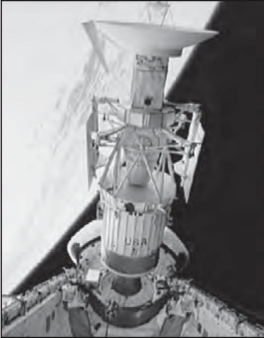
*Magellan spacecraft and attached Inertial Upper Stage (IUS) rocket being released into a temporary Earth orbit from the payload bay of the space shuttle orbiter Atlantis on May 4, 1989. Shortly afterward, the IUS propelled the spacecraft on a Sun-looping trajectory toward Venus, where it arrived on Aug. 10, 1990. NASA/JPL*
