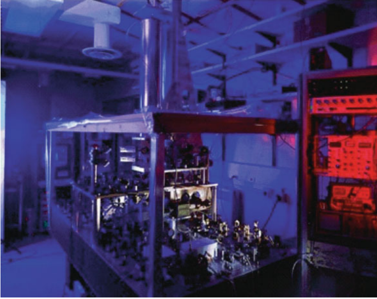
Fig. 6.9 The modern alternative to the sundial, clepsydra, or the pendulum clock – the NIST-F1 Cesium Fountain atomic clock, which provides the most accurate time standard available in the world, and keeps time to within better than one part in a thousand trillion (image courtesy of NIST)
