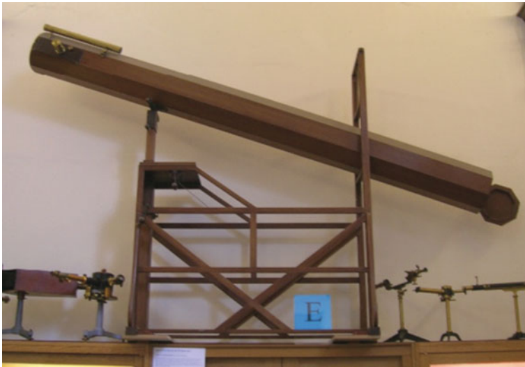
Fig. 9.13 William Herschel's 10-foot telescope from 1790, which featured a 9-in. diameter mirror and controls to move the telescope vertically and laterally. Herschel made this telescope himself, and used it to discover hundreds of new objects, including galaxies and comets with his sister Caroline (photograph by the author, from Cambridge University Whipple Museum of Science)
