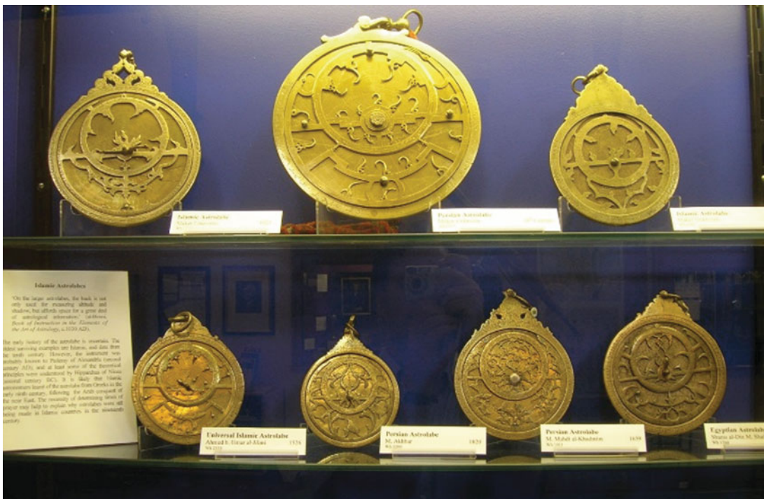
Fig. 8.19 A display of Persian and Arabic astrolabes from the fifteenth to the eighteenth centuries, from the Cambridge Museum of Science and Technology. Such devices were used by Islamic navigators to sight stars and to find the time and directions anywhere on the Earth from the stars (photo by the author)
