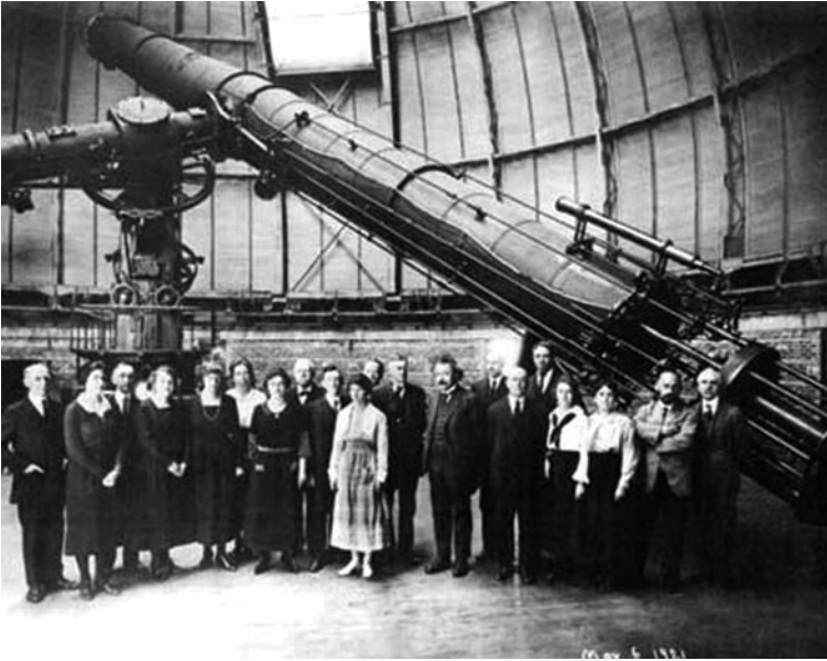
Fig. 9.18 The Yerkes 40" refractor, Hale's first largest telescope in the world, completed in 1897, and still the world's largest refracting (lens-based) telescope. The telescope was famous enough to attract a very well-known visitor, Albert Einstein, shown in the center of this 1921 photo ( image source: http://commons.wikimedia.org/wiki/File:Yerkes_Observatory_Astro4p7.jpg )
