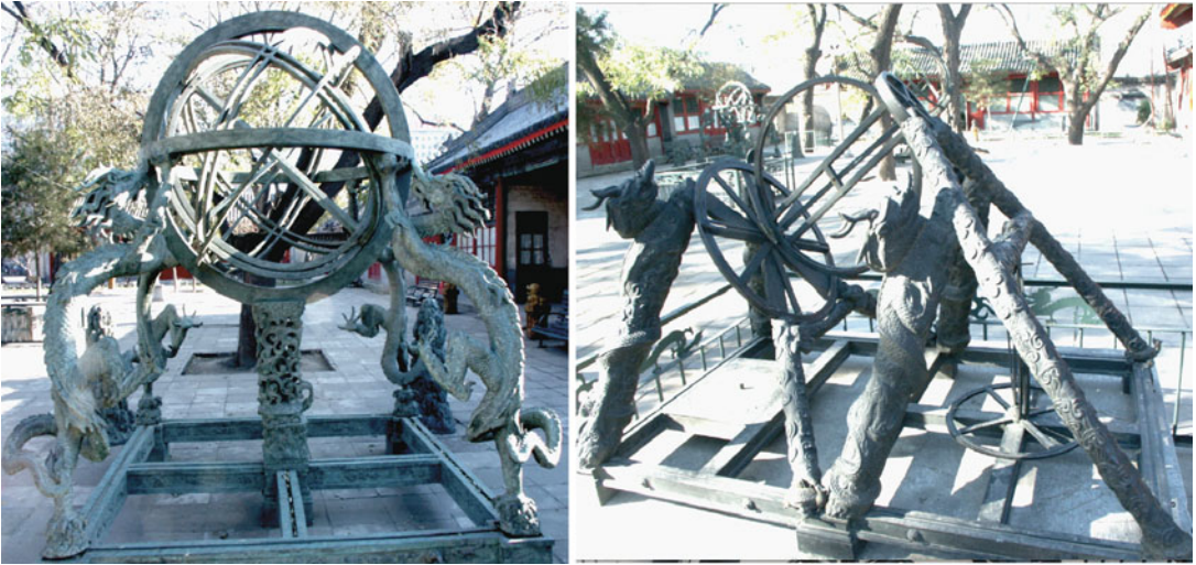
Fig. 5.18 Chinese astronomical instruments at the Nanjing Purple Mountain Observatory. ( Left ) An armillary sphere from the 15th century, used for astronomical calculations, and ( right ) a simplified armilla from 1439, which is designed much as a modern equatorial telescope mount for visual observations of stars and planets. These instruments are decorated with the dragons associated with the cardinal directions and were used at one of many of the professional astronomical bureaus in ancient China that provide some of the most sophisticated observational data of any historical civilization (photographs by William Smith, reprinted with permission)
