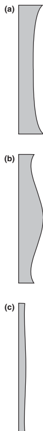
Fig. 6.7 Shapes of the Schmidt corrector: (a) shows a plate whose power decreases radially, starting with zero power at center; (b) shows a plate with positive power at center, decreasing to zero at 0.866 fractional radius; and (c) shows the actual cross-section of a corrector with shape (b) for an f/3 system.
