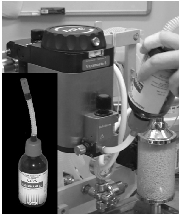
Fig 4.9 Filling an MIE halothane vaporiser using a keyed filler. The halothane bottle with the filler attached is shown in the inset.
