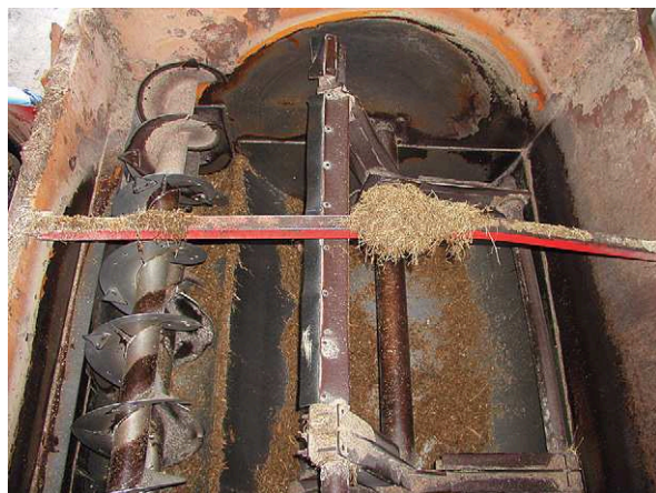
Figure 5-10 There are many designs of mechanical feed mixers. In this case a paddle does most of the mixing while the screw delivers the final mix. The efficiency of any mixer depends on the operator mixing consistently and according to the instructions of the manufacturer. (Courtesy of K Nordlund)
