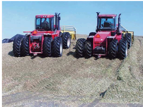
Figure 5-15 These heavy units compact the silage very effectively, reducing air pockets to a minimum. Good compression reduces the necessity for chopping the crop too small. Good particle size is essential for proper digestion. (Courtesy of K Nordlund)
