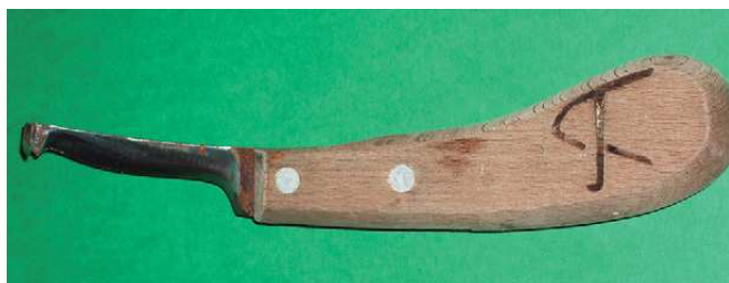
Figure 14-57 This is an older model Swedish knife. The edge of the narrower blade show signs of considerable wear. Note that Figures 14-56 and 14-57 are a matched pair of left- and right-handed knives. (Courtesy of A Brizzi)
