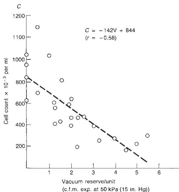
**Fig. 25.2** Relationship between mean cell count of herd bulk milk (C) and vacuum reserve per unit (V). Source: Nyhan & Cowhig (1967).
