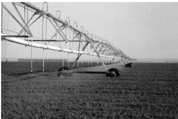
Fig. 71.1 A centre pivot irrigation system.
