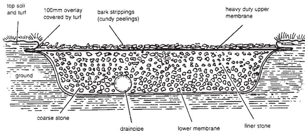
Fig. 31.11 Cross-section of a cow track.
