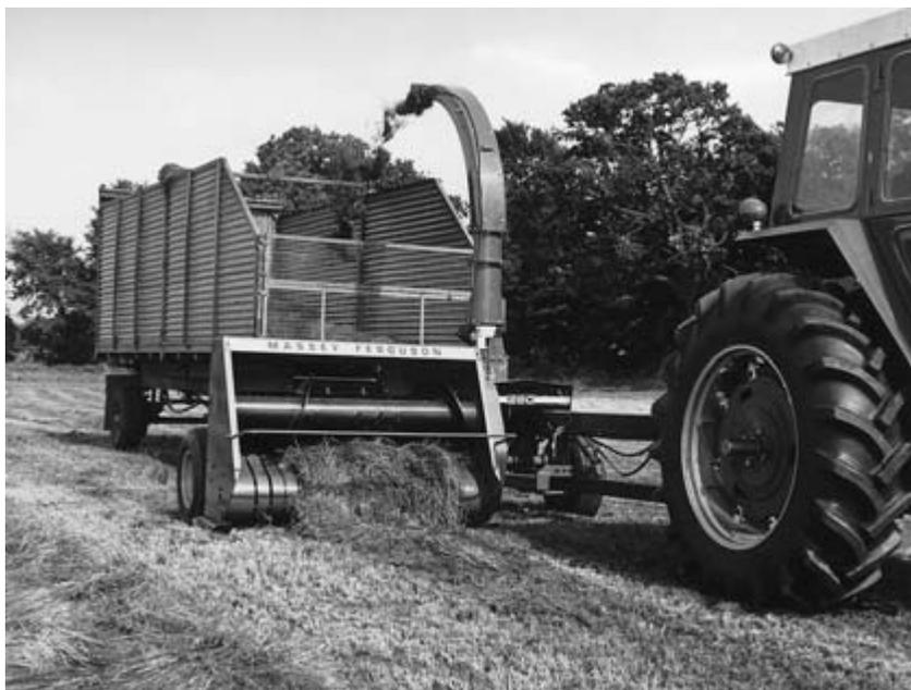
**Fig. 4.13** Silage making with a precision chop forage harvester.
