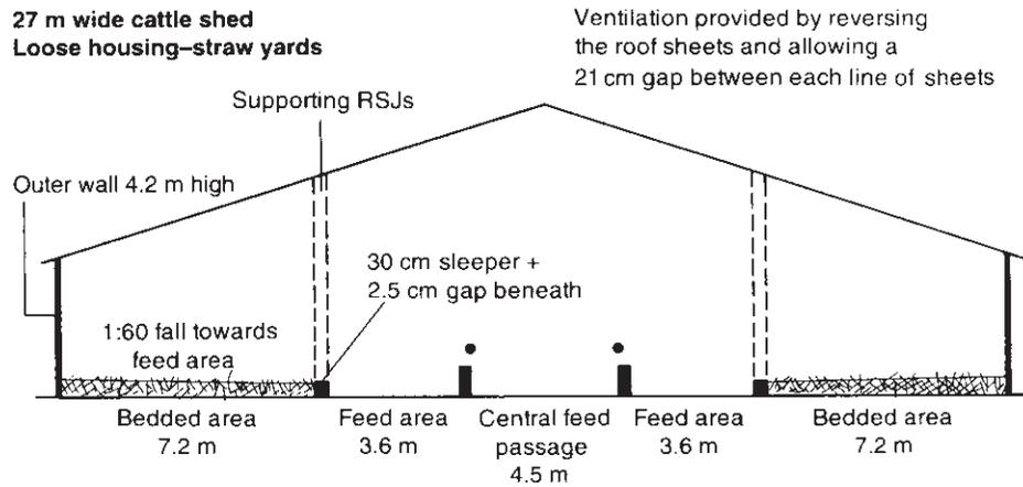
**Fig. 4.24** A 27.5 m (90 ft) wide cattle shed with loose housing (reprinted from Hughes, 2000).
