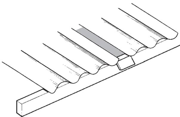
**Fig. 56.9** The 'breathing' roof: ventilation achieved by leaving a gap between the roof sheets.
