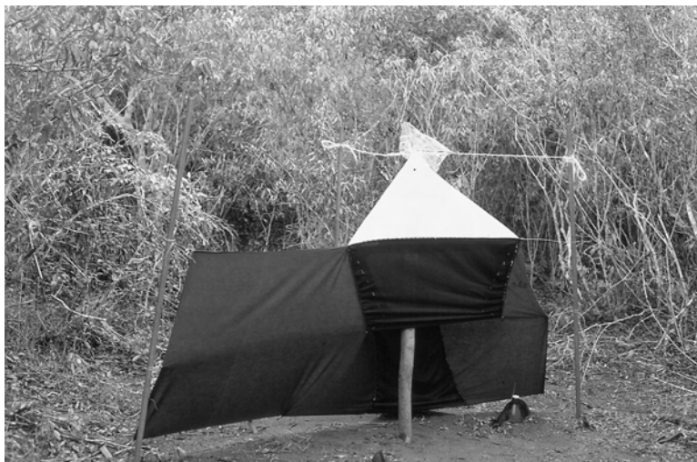
Fig. 5. A Ngu tsetse-fly trap, devised by R. Dransfield, and used in the control of animal trypanosomiasis in Kenya (courtesy of A.M. Jordan).
