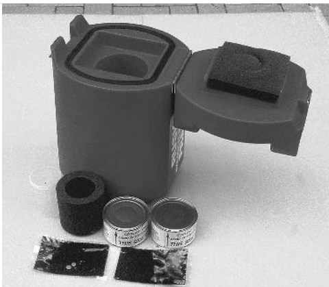
Fig. 20.7. The component parts of the Equitainer. The ballast bags can be seen in the foreground; behind them are the two coolant cans or blocks and to their left the black foam insulating jacket (which acts as a thermal impedance pad and foam-rubber protective padding) into which the plastic semen container (isothermalizer) – far left – is placed. (From Hamilton-Thorn Research, Danvers, Massachusetts.)
