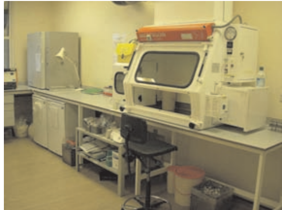
Figure 18.6 View of a CL3 laboratory, showing the exhaust protective cabinet that provides safety to the operator while manipulating cultures containing hazardous pathogens.
