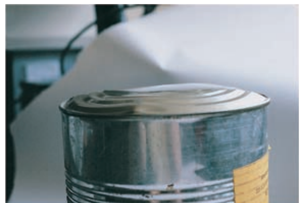
Figure 8.15 A 'blown' can of hazelnut purée that had not been properly heat-treated, resulting in the formation of botulinum toxin type b; 27 people developed botulism after eating hazelnut yoghurt prepared from the contents of such a can. Courtesy of Dr Richard Gilbert, Central Public Health Laboratory.
