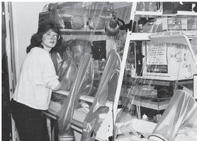
Figure 23.2 Negative-pressure filter isolator for high-security laboratory work. This laboratory contains an incubator, an automated blood count machine, a cassette-based biochemistry analyser, a coagulometer, a blood mixer, a microscope and a centrifuge in a bench area of 2 m 2 .
