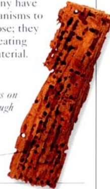
larval feeding tunnels damage timber
