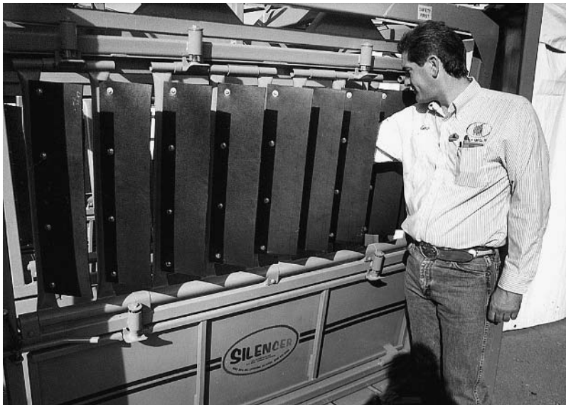
Fig. 7.7. Rubber louvres installed on the squeeze slide to prevent incoming cattle from seeing people.
