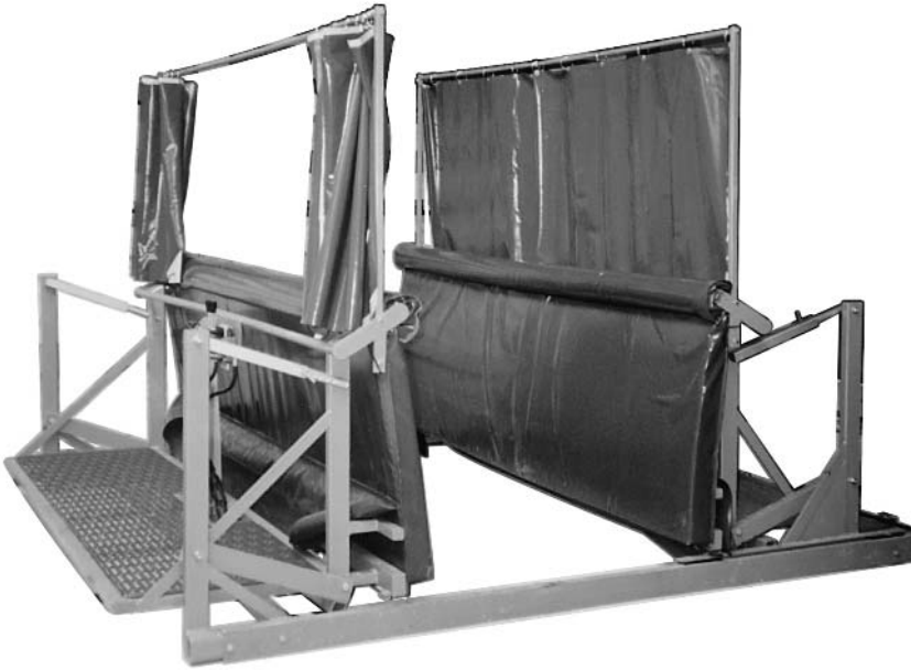
Fig. 17.5. (a) A hydraulically operated deer handler shown in its open position; this creates a small padded room about 1.4 m × 2.6 m long which is suitable for holding one or two deer. The curtains are closed during loading but can be opened after the animal(s) has (have) been restrained. The operator works from the small platform and restrains an animal by operating the moving wall, and applying steady pressure to the animal aligned between the two walls. ( Continued overleaf. )
