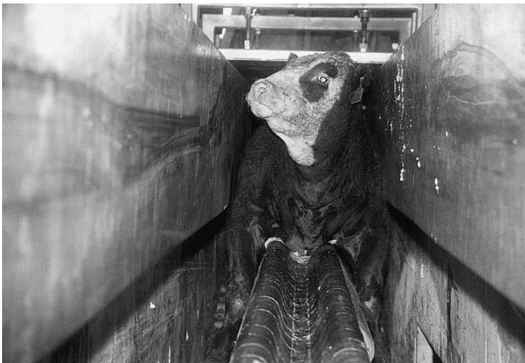
Fig. 20.9. Large steer in the double-rail (centre-track) restrainer. Note that the conveyor is shaped to fit the animal's brisket.
