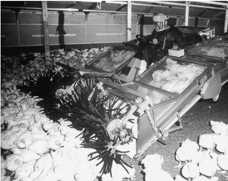
Fig. 18.1. Automated broiler harvester. Photo courtesy of Anglia Autoflow.
