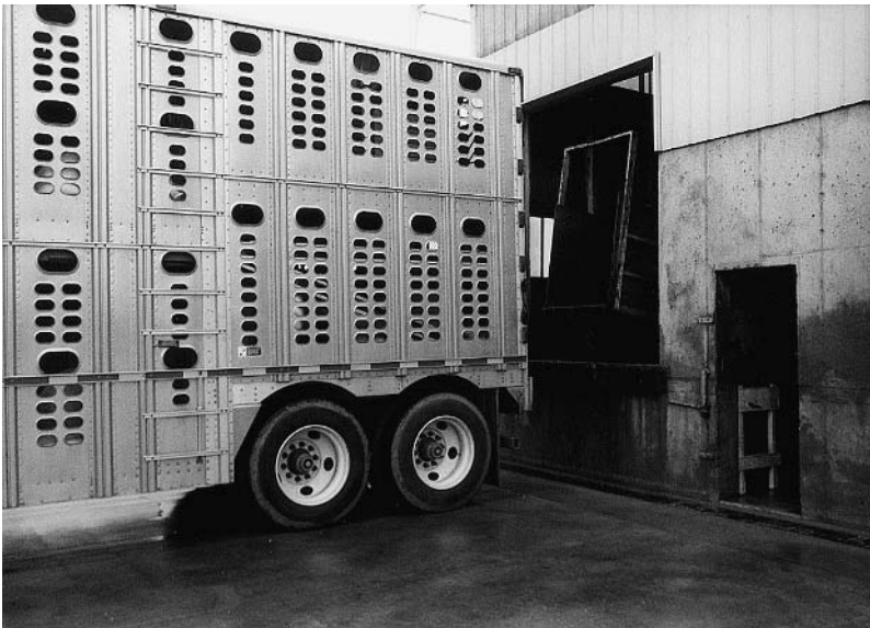
Fig. 9.2. Typical aluminium-sided trailer which is used in the USA for transporting both cattle and pigs. Numerous holes provide abundant ventilation.
