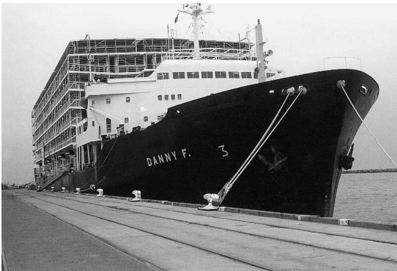
Fig. 1.1. Huge ships with multiple decks of sheep pens transport millions of sheep from Australia to the Middle East. Large ships hold 60,000–100,000 sheep.
