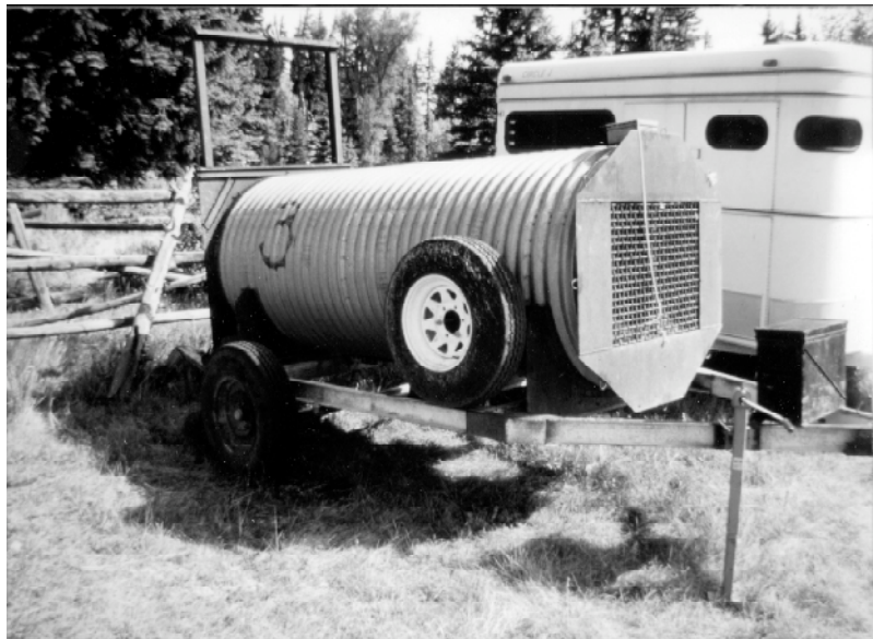
Figure 15–6 A culvert trap baited with garbage is used to capture bear. (Courtesy of R. Grogan.)
