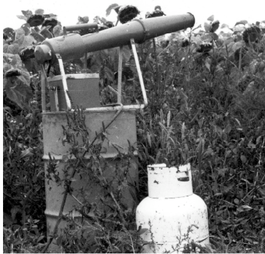
Figure 22-10 Noise device used for controlling blackbirds. (Courtesy of the U.S. Fish and Wildlife Service.)
