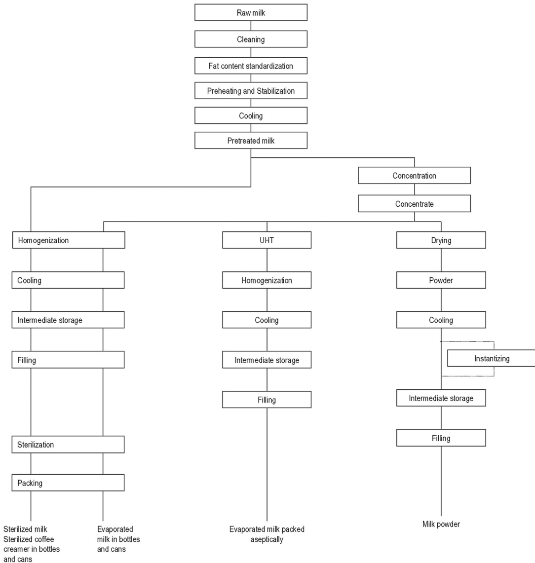
Figure 2.36. Flowchart for manufacture of evaporated and powdered milk along with sterilized fluid milk processing procedures. Adapted from E. Spreer (106).
