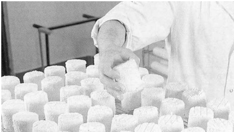
Figure 2.30b. Drying processes for the soft goat cheeses after removal from the plastic cheese hoops. Source: Goat milk cheese plant, Poitiers, France.
