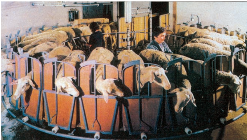
Figure 3.11. Typical rotary milking parlor for dairy sheep. Photo: F. Kervina et al., 1981, by permission, Alfa-Laval Co. Publ., Tumba, Sweden.
