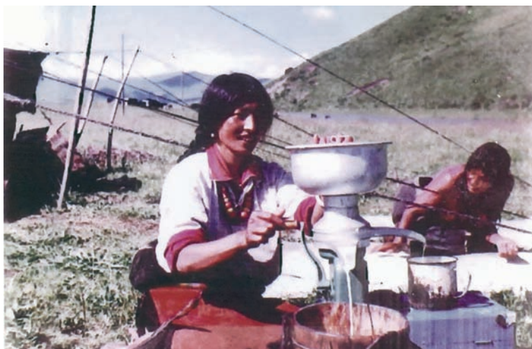
Figure 7.2. A mechanical milk separator for cream separation. Photo provided by Yucai Zheng.
