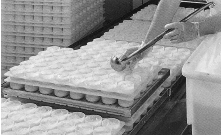
Figure 2.30a. Transfer of soft curd body of goat milk cheese to the plastic hoops for draining whey in a French commercial goat milk cheese plant. Source: Goat milk cheese plant, Poitiers, France.
