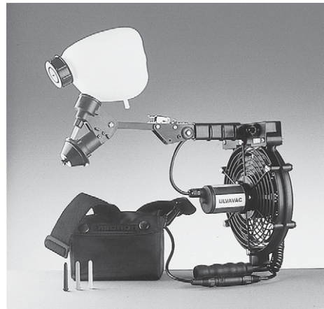
Fig. 5.2 Ulvavac fan sprayer for spray vaccination on the farm. (Courtesy of Micron Sprayers Ltd, UK.)
