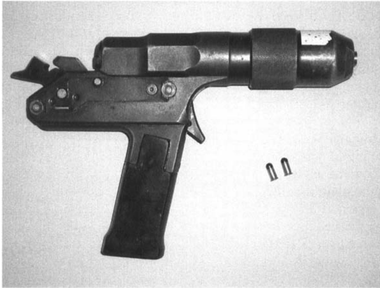
Figure 8.4 'Cash' captive bolt pistol with cartridges used to propel the bolt.
