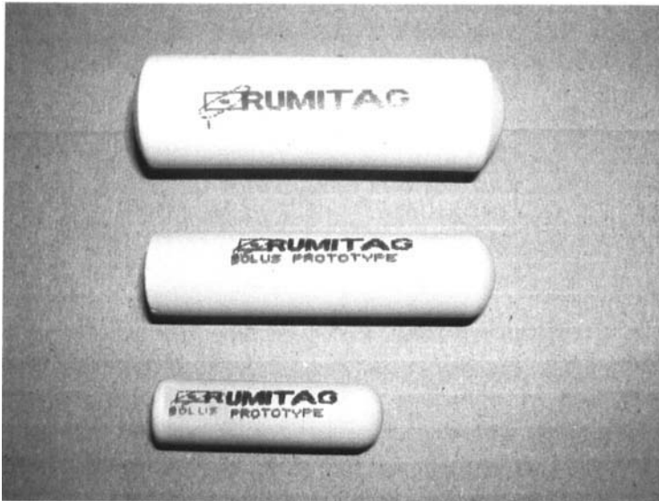
Fig. 7.32 Electronic identification rumen boluses for cattle and sheep (picture by Shearwell Data Ltd).
