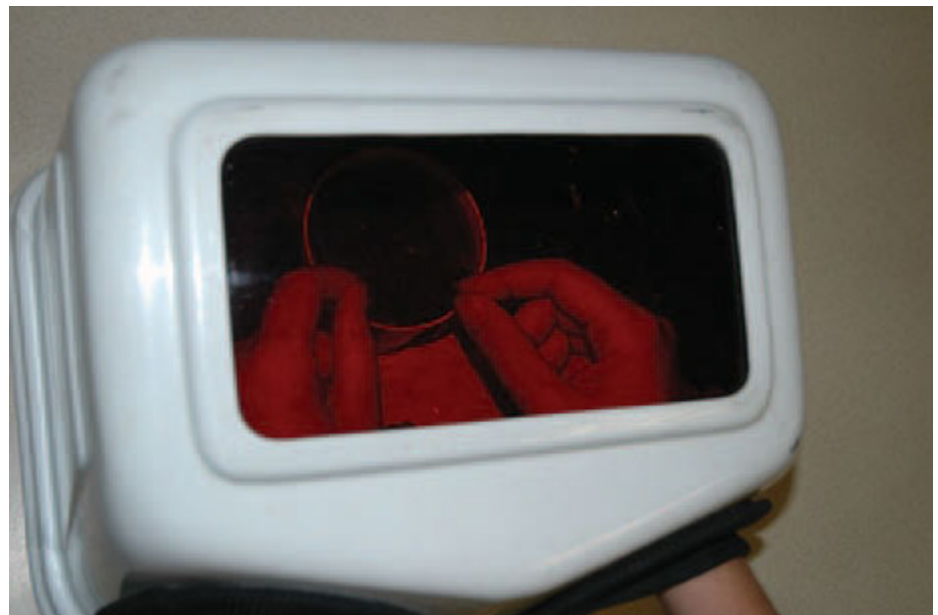
Figure 4.24 The red 'window' provides 'safe' light within the processor allowing visualisation of the process.
